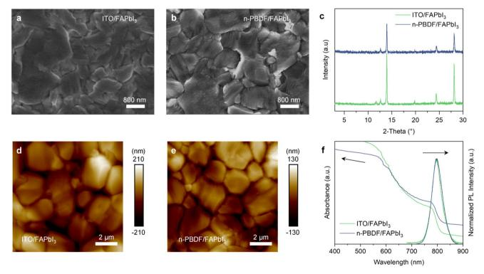
Fig. 2 SEM images of perovskite (FAPbl<sub>3</sub>) grown on (a) ITO and (b) n-PBDF electrodes on the glass substrate. (c) XRD spectra of perovskite grown on the ITO and n-PBDF electrodes. AFM height images of perovskite grown on the (d) ITO and (e) n-PBDF electrodes. (f) UV-vis and PL spectra of perovskite grown on ITO and n-PBDF electrodes.
