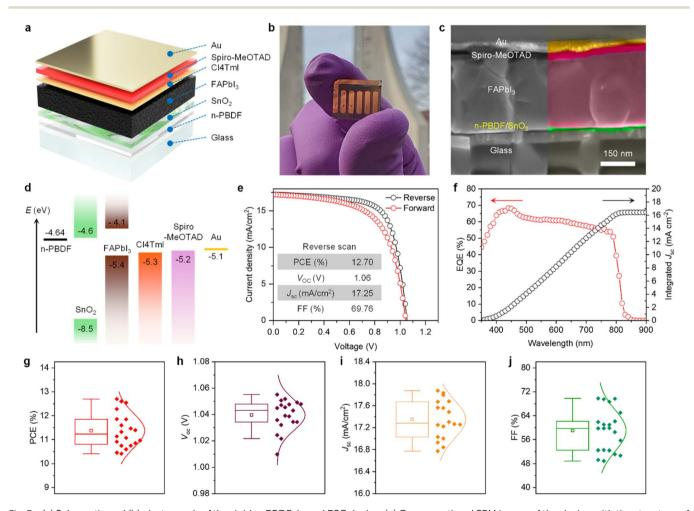
Fig. 3 (a) Schematic and (b) photograph of the rigid n-PBDF-based PSC device. (c) Cross-sectional SEM image of the device with the structure of glass/n-PBDF/SnO<sub>2</sub>/perovskite (FAPbl<sub>3</sub>)/Cl4Tml/spiro-MeOTAD/Au. (d) Energy band alignment of the component layers in the n-PBDF-based PSC. (e) J-V characteristics and (f) EQE with corresponding integrated  $J_{sc}$ . (g-j) Statistical results of the rigid n-PBDF-based PSC devices (from three batches, n = 20).
