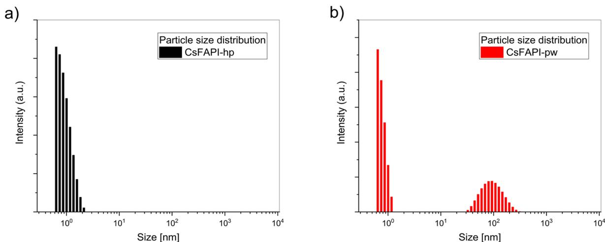
Fig. 2 Particle size distribution for CsFAPbI<sub>3</sub>-hp (a) and CsFAPbI<sub>3</sub>-pw solution, and (b) measure by dynamic light scattering technique.
