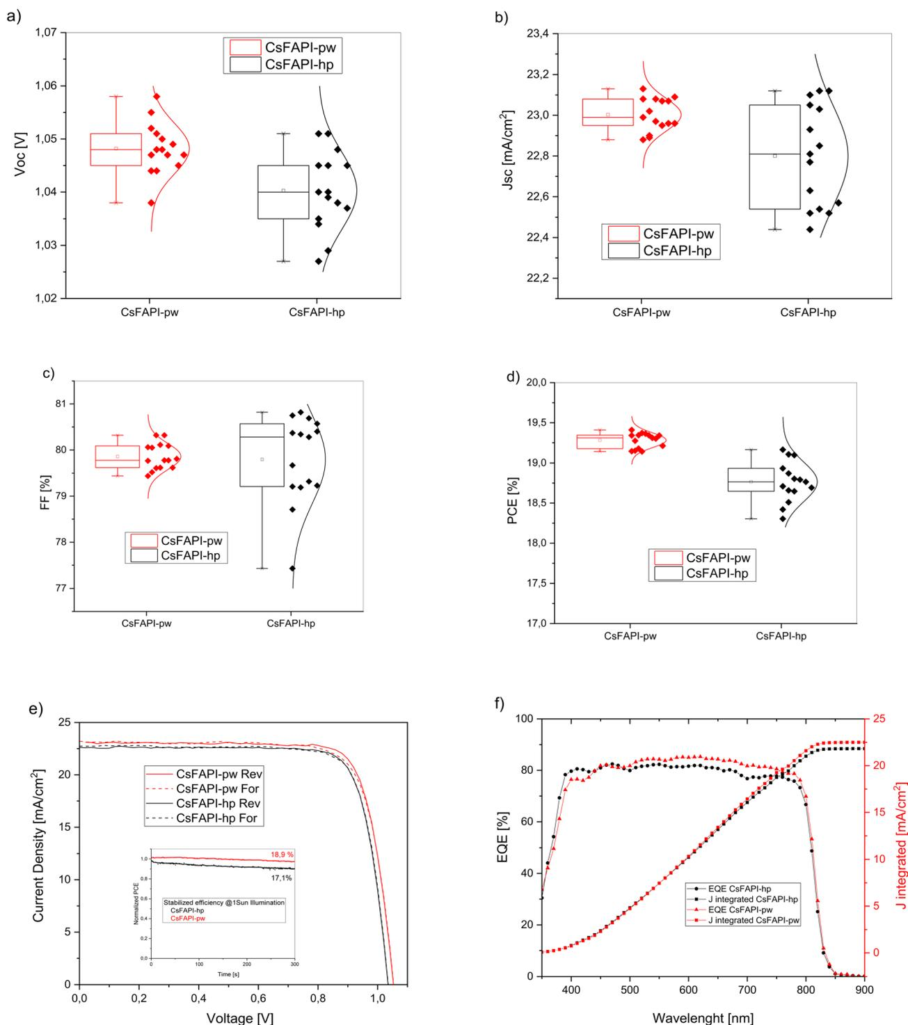
Fig. 4 Statistics of photovoltaic parameters for CsFAPi-hp and CsFAPi-pw devices:  $V_{oc}$  (a)  $J_{sc}$  (b) FF (c) and PCE (d);  $J$ - $V$  curves for the record devices of CsFAPi-hp and CsFAPi-pw respectively on 0.5 cm<sup>2</sup> active area (e); EQE of the best devices (f).
