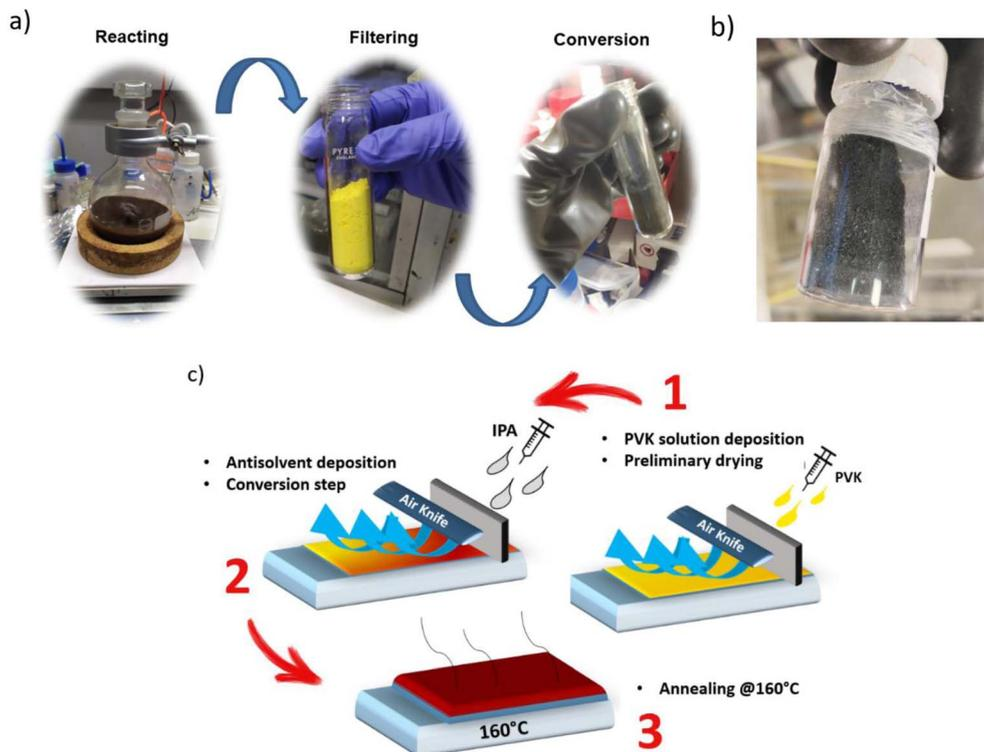
Fig. 1 CsFAPbI<sub>3</sub> powder synthesis steps (a); black CsFAPbI<sub>3</sub> powder (b); process routine for CsFAPbI<sub>3</sub> perovskite deposition in ambient air with blade coating technique (c).
