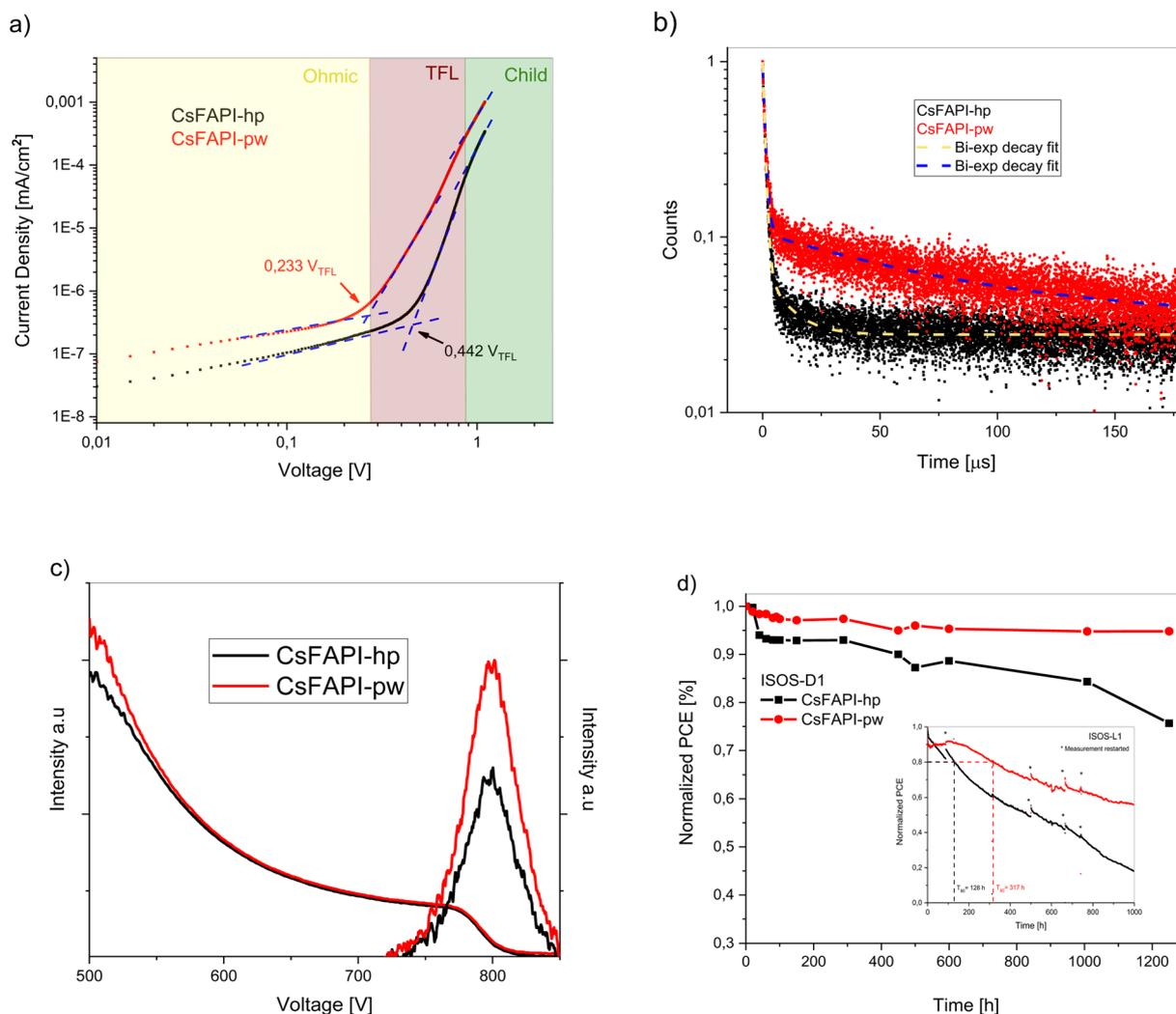
**Fig. 5** SCLC analysis (a), transient photoluminescence decay (b), UV-Visible spectra and PL measurements of PVK films (c) and ISOS-D1 at 30% RH in UV-filtered box for CsFAPi-hp and CsFAPi-pw (d), respectively.
