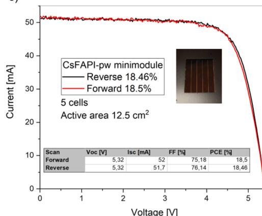
Fig. 6 Minimodule Image and EDX analysis of P1–P2–P3 scribing process (scale bar is 250  $\mu\text{m}$ ) (a); cross view of P1/P2/P3 process in stack and dead area (b)  $I$ – $V$  curve of the best minimodule made with CsFAPbI<sub>3</sub>-pw precursor (c).
