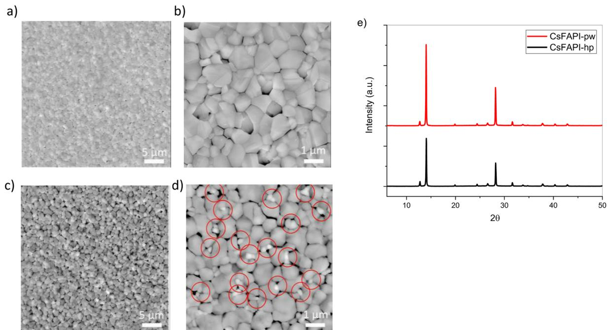
Fig. 3 SEM top view of CsFAPbI<sub>3</sub>-pw (a and b) and CsFAPbI<sub>3</sub>-hp (c and d) at lower and higher magnification, respectively; red circles in Fig. 2d highlight unreacted PbI<sub>2</sub>; XRD diffraction pattern of CsFAPbI<sub>3</sub>-hp and CsFAPbI<sub>3</sub>-pw deposited by blade coating on bare FTO (e).
