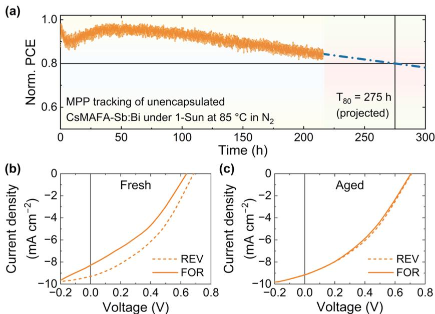
Fig. 7 (a) MPP tracking of a CsMAFA-Sb:Bi (unencapsulated) device (2.4% initial PCE) under 1-Sun illumination at 85 °C under N<sub>2</sub> atmosphere. The  $T_{80}$  value was predicted by extrapolating the experimental data.<sup>83</sup> The  $J$ - $V$  curves of the device are shown (b) before and (c) after the tracking.
