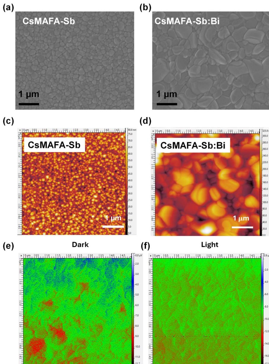
Fig. 2 (a and b) SEM images and (c and d) AFM images of CsMAFA-Sb and CsMAFA-Sb:Bi films on FTO/c-TiO<sub>2</sub>. Surface potential measurements of CsMAFA-Sb:Bi film in (e) dark and under (f) light illumination.
