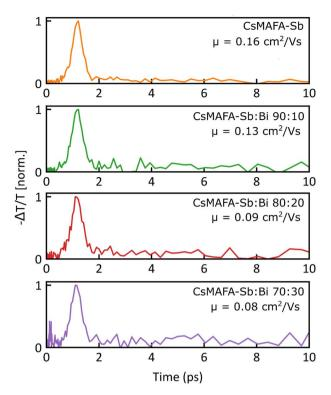
Fig. 4 Normalized photoinduced THz conductivity transients measured for (a) reference CsMAFA-Sb (b) target CsMAFA-Sb:Bi (90: 10) (c) CsMAFA-Sb:Bi (80: 20) and (d) CsMAFA-Sb:Bi (70: 30) thin films after 3.1 eV pulsed excitation. The values for the initial electron–hole sum mobility extracted from the peak of the photoconductivity (based on the methodology described in Note 3, ESI†) are reported on the figures.
