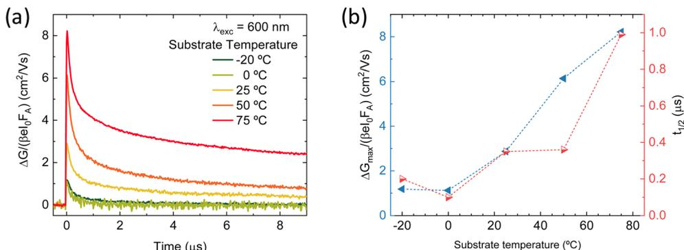
Fig. 3 (a) Comparison of TRMC traces of a series of perovskite films vapor-deposited with varying substrate temperature, recorded at 600 nm excitation at the same fluence of  $6 \times 10^{10}$  photons per cm<sup>2</sup> per pulse. (b) Summary of maximum effective mobility (blue, left) and half lifetime (red, right) extracted from the TRMC traces.
