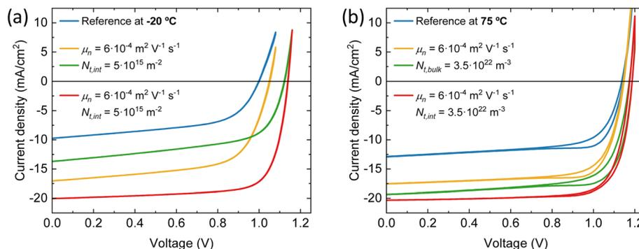
Fig. 6 Simulated  $J$ - $V$  curves at 1 sun eq. at (a)  $-20$  °C substrate temperature for different electron mobility and trap density at both interfaces (b)  $75$  °C substrate temperature for different electron mobility and bulk trap density.
