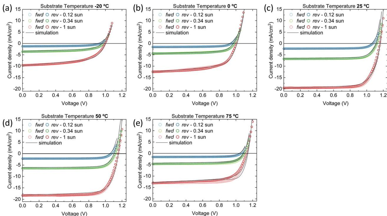
**Fig. 5**  $J$ - $V$  characteristics of the vacuum deposited wide bandgap perovskite solar cells for multiple light intensities and at (a) -20 °C (b) 0 °C (c) 25 °C (d) 50 °C and (e) 75 °C substrate temperatures. The open symbols represent the experimental data; the solid lines the simulations. First the forward scan from  $V_{\text{min}}$  to  $V_{\text{max}}$  is performed and afterwards the backward scan from  $V_{\text{max}}$  to  $V_{\text{min}}$ .
