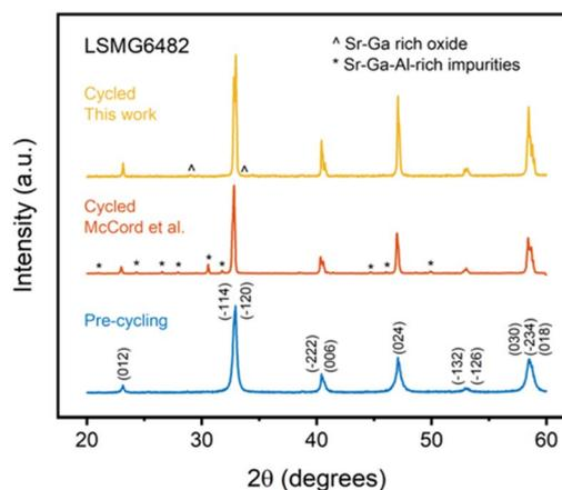
Fig. 3 XRD patterns of LSMG6482 before cycling, after cycling from a  $p\text{O}_2$  of  $10^{-3}\text{ atm}$  to  $10^{-4}\text{ atm}$  (McCord *et al.*), and after cycling from a  $p\text{O}_2$  of  $10^{-4}\text{ atm}$  to  $10^{-7}\text{ atm}$ . LSMG6482 forms in the perovskite structure with no secondary phases prior to cycling. Cycling causes Sr–Ga rich secondary phases to form in the material.
