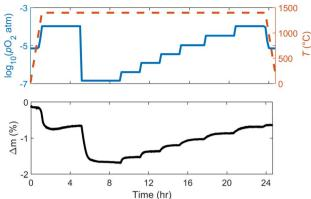
Fig. 1 Thermogravimetric results for LSMG6482 at T = 1400 °C. Input conditions are shown on the top plot while mass response is shown on the bottom plot.
