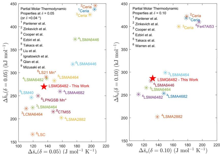
Fig. 7 Comparison of  $\Delta \bar{h}_o(\delta)$  and  $\Delta \bar{s}_o(\delta)$  at  $\delta = 0.05$  (left) and  $\delta = 0.10$  (right) LSMG6482 and notable perovskites from literature. Insights from Ellingham diagram.
