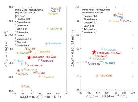
Fig. 7 Comparison of  $\Delta \bar{h}_{o}(\delta)$  and  $\Delta_{o}\bar{s}(\delta)$  at  $\delta=0.05$  (left) and  $\delta=0.10$  (right) LSMG6482 and notable perovskites from literature. Insights from Ellingham diagram.
