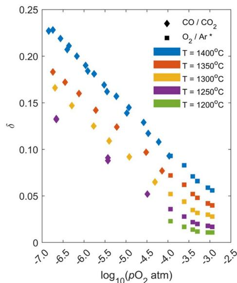
Fig. 2 Measured equilibrium  $\delta$  from thermogravimetric experiments for LSMG6482 as a function of temperature and  $p\text{O}_2$ . Diamond markers are from this study, while square markers (marked \* in legend) are from McCord *et al.*
