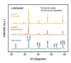
Fig. 3 XRD patterns of LSMG6482 before cycling, after cycling from a  $pO_2$  of  $10^{-3}$  atm to  $10^{-4}$  atm (McCord *et al.*), and after cycling from a  $pO_2$  of  $10^{-4}$  atm to  $10^{-7}$  atm. LSMG6482 forms in the perovskite structure with no secondary phases prior to cycling. Cycling causes Sr-Ga rich secondary phases to form in the material.
