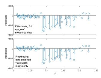
Fig. 5 Residuals of the oxygen defect model when fitted to the full thermogravimetric data set (top) compared to those when fitted to only data achieved through trace oxygen mixing (bottom).
