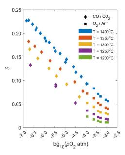
Fig. 2 Measured equilibrium  $\delta$  from thermogravimetric experiments for LSMG6482 as a function of temperature and pO2. Diamond markers are from this study, while square markers (marked \* in legend) are from McCord et al.
