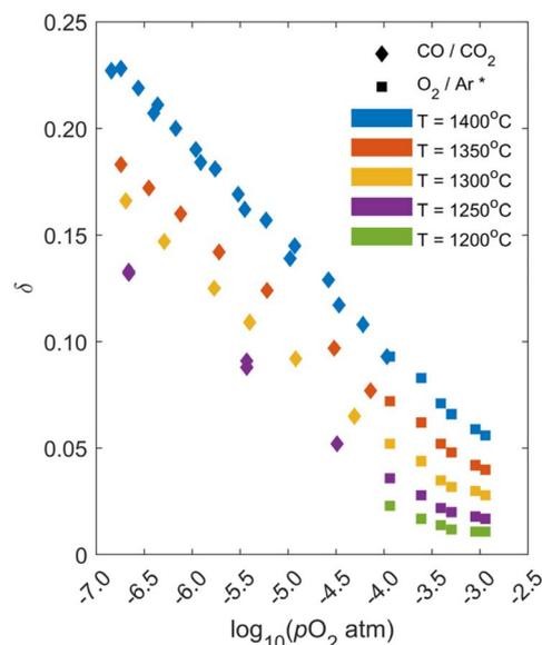
Fig. 2 Measured equilibrium  $\delta$  from thermogravimetric experiments for LSMG6482 as a function of temperature and  $p\text{O}_2$ . Diamond markers are from this study, while square markers (marked \* in legend) are from McCord *et al.*
