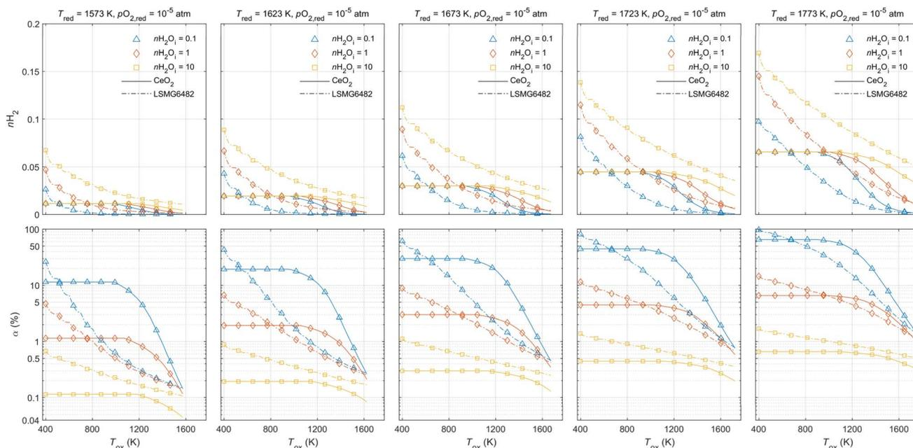
Fig. 9  $H_2$  yield (top row) and steam conversion (bottom row) for  $T_{red}$  ranging from 1573 K to 1773 K at  $p_{O_2,red} = 10^{-5}$  atm for ceria and LSMG6482 under fixed steam inputs and variable  $T_{ox}$ . Solid lines represent results for ceria, while dashed-dotted lines represent results for LSMG6482.
