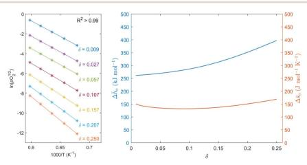
$ln(pO_2^{1/2})$  vs. 1000/T fits at select  $\delta$  (left) and partial thermodynamic properties of LSMG6482 as a function of delta (right).
