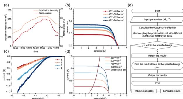
Fig. 6 Simulation model construction. (a) Variation of daily irradiation intensity and PV operating temperature. (b) ISDM PV  $I$ - $V$  characteristic curve. (c)  $I$ - $V$  characteristic curve of electrolytic cell set with different number of electrolytic cells connected to it. (d) Variation of working point of electrolytic cell set under different specifications of PV module working conditions. (e) Schematic diagram of the operation logic of the coupled control model.
