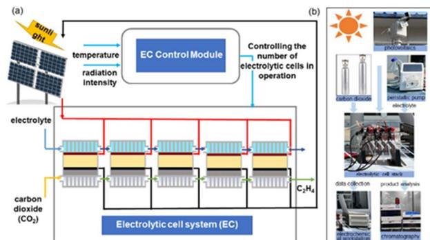
Fig. 3 (a) Schematic diagram of a photovoltaic-driven electrocatalytic carbon dioxide reduction electrolysis cell system; (b) physical diagram of the carbon dioxide reduction stack and test platform.
