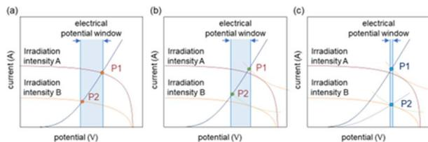
Fig. 1 Schematic diagram of system  $I$ - $V$  characteristics for different connection methods (a) direct coupling (b) indirect coupling (c) this working design method (d) comparison of selective performance of electrolytic cell for carbon monoxide under different control modes.
