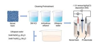
Fig. 2 Ni<sub>3</sub>Fe(OH)<sub>9</sub> anode preparation steps.
