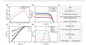
Fig. 6 Simulation model construction. (a) Variation of daily irradiation intensity and PV operating temperature. (b) ISDM PV I-V characteristic curve. (c) I-V characteristic curve of electrolytic cell set with different number of electrolytic cells connected to it. (d) Variation of working point of electrolytic cell set under different specifications of PV module working conditions. (e) Schematic diagram of the operation logic of the coupled control model.
