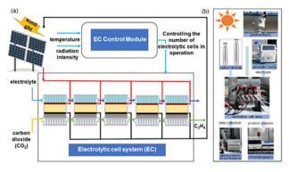
Fig. 3 (a) Schematic diagram of a photovoltaic-driven electrocatalytic carbon dioxide reduction electrolysis cell system; (b) physical diagram of the carbon dioxide reduction stack and test platform.
