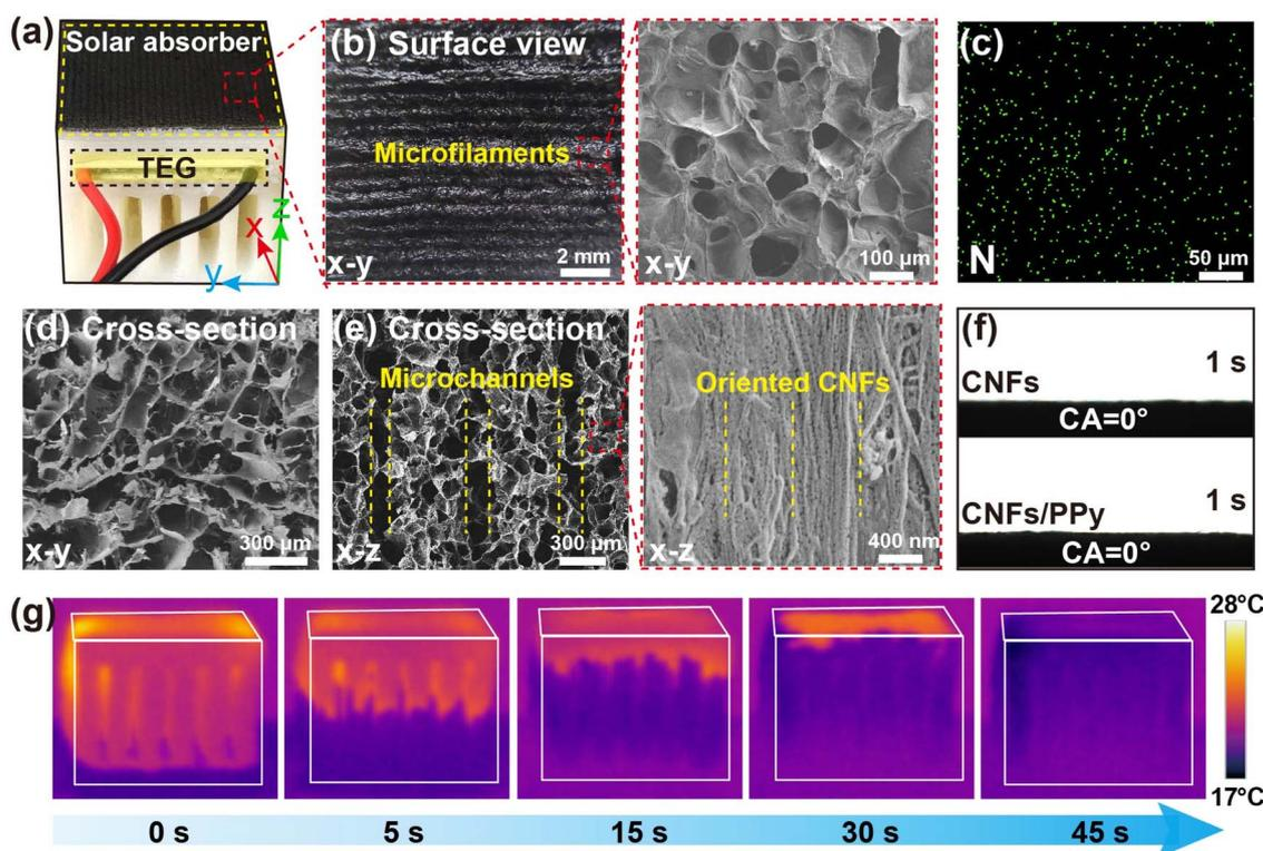
**Fig. 3** (a) Digital photograph of the heatsink-like SG-TEG hybrid device. (b) Surface macro photograph (left) and a local SEM image (right). (c) EDS image of the characteristic element. (d) SEM images of the transverse cross-sections. (e) SEM images of the longitudinal cross-sections. (f) Surface contact angle measurements. (g) Water diffusion characterization over 45 s.
