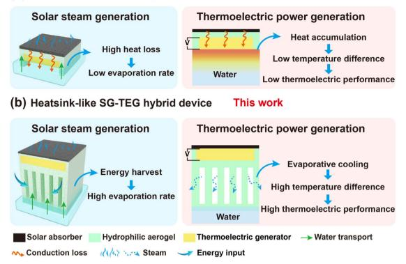
Fig. 1 Schematic illustration of synergistic interfacial evaporation and thermoelectric power generation based on (a) a conventional SG-TEG hybrid device and (b) a heatsink-like SG-TEG hybrid device.
