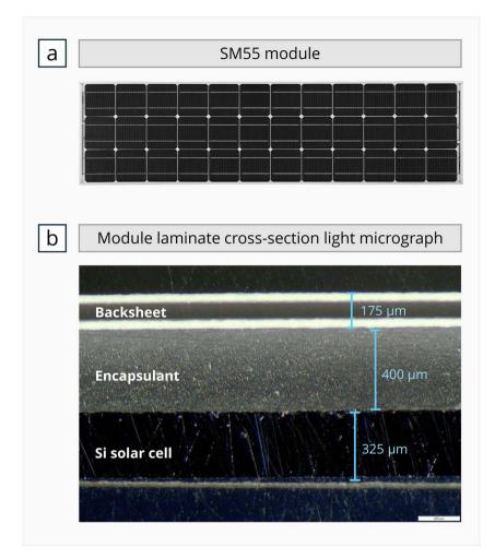
Fig. 3 (a) Photograph of a Siemens SM55 module. (b) Light micrograph of the cross section of part of the module laminate: 3-layer backsheet, back encapsulant and Si-solar cell.
