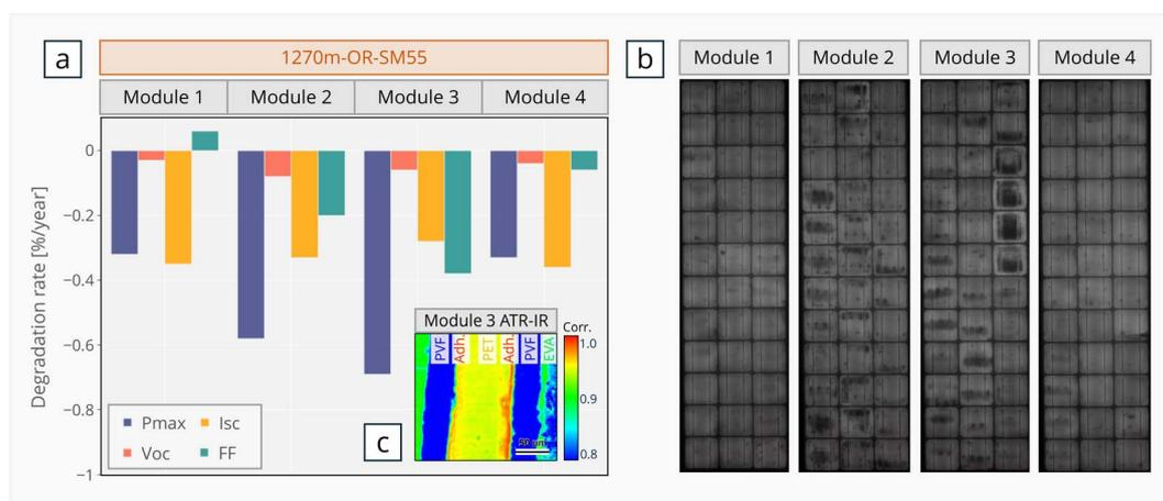
Fig. 10 (a) Degradation rates of the module  $I$ - $V$  parameters (indoor) and (b) EL images of four modules from the 1270m-OR-SM55 system. (c) ATR-IR image, shown as an inset in the figure, highlights the dark area of Module 3 with compare-correlation analysis with the IR spectrum of the unaged adhesive.
