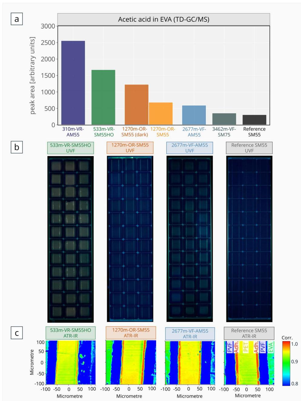
**Fig. 11** (a) Amount of acetic acid detected in the EVA with TD-GC/MS. (b) UVF images of the modules after 30 years of outdoor exposure, alongside a UVF image of a non-weathered reference SM55 module. (c) ATR-IR images of the cross-sections of backsheets after compare-correlation with the IR spectrum of the unaged adhesive (high correlation = red).
