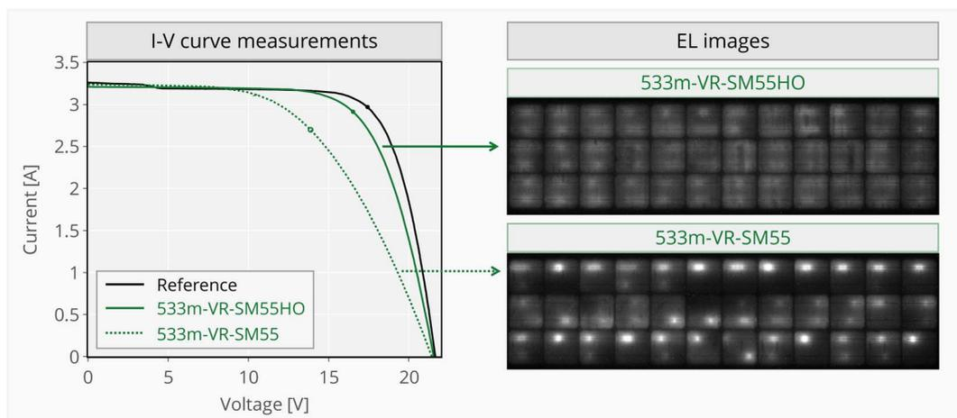
**Fig. 7**  $I-V$  curves of the reference, SM55, and SM55-HO modules from the 533m-VR-SM55(HO) site, along with EL images taken after approximately 30 years of outdoor operation. The SM55 module exhibits increased series resistance and reduced fill factor due to recurring solder bond failures, visible as dark areas near cell edges and bright spots along the ribbons in the EL images.
