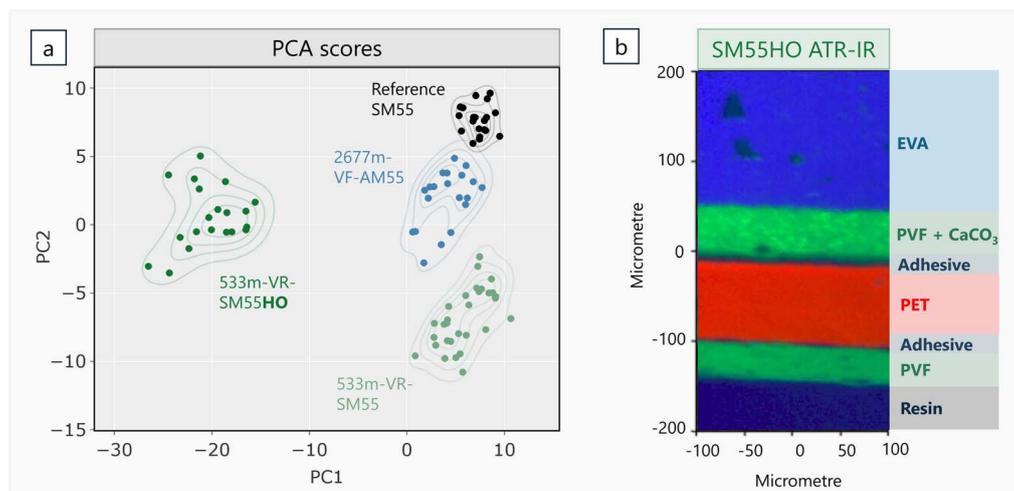
Fig. 8 (a) PCA scores obtained from PCA clustering analysis of the whole NIR spectra, highlighting a clear distinction of the SM55-HO module type. (b) ATR-IR image of the cross-section of the backsheet of a SM55-HO module showing the  $\text{CaCO}_3$  filler.
