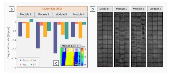
Fig. 10 (a) Degradation rates of the module I-V parameters (indoor) and (b) EL images of four modules from the 1270m-OR-SM55 system. (c) ATR-IR image, shown as an inset in the figure, highlights the dark area of Module 3 with compare-correlation analysis with the IR spectrum of the unaged adhesive.
