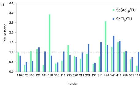
Fig. 5 (a) Relative intensity and (b) texture coefficients for different (hkl) planes of Sb<sub>2</sub>S<sub>3</sub> films from Sb(Ac)<sub>3</sub>/TU and SbCl<sub>3</sub>/TU precursor solutions.
