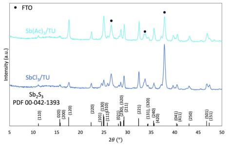
Fig. 4 X-ray diffractograms of Sb<sub>2</sub>S<sub>3</sub> films from Sb(Ac)<sub>3</sub>/TU (turquoise) and SbCl<sub>3</sub>/TU (dark blue) solutions.
