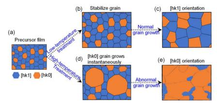
Fig. 2 Mechanism of  $Sb_2S_3$  orientation dependence on grain growth. Surface texture of (a) the  $Sb_2S_3$  precursor film, (b) the  $Sb_2S_3$  precursor film after stabilization at low temperature, and (c) after normal grain growth. (d) and (e) The surface textures of the  $Sb_2S_3$  film after thermal treatment at high temperature and then subjected to abnormal grain growth. Reproduced with permission from ref. 8 Copyright 2024, RSC.
