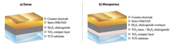
Fig. 8 Scheme of (a) dense and (b) mesoporous architectures of Sb<sub>2</sub>S<sub>3</sub> devices.
