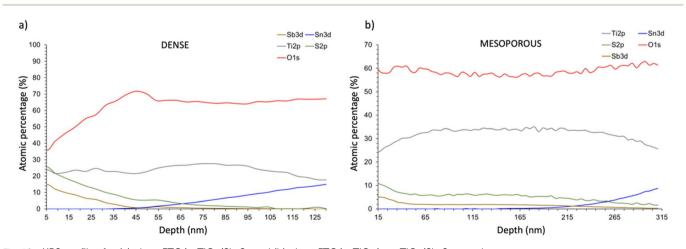
Fig. 10 XPS profiles for (a) glass-FTO/c-TiO $_2$ /Sb $_2$ S $_3$  and (b) glass-FTO/c-TiO $_2$ /mp-TiO $_2$ /Sb $_2$ S $_3$  samples.
