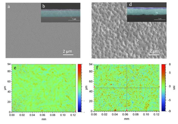
Fig. 3 SEM micrographs in top-view and cross-section (inset) of (a and b) Sb(Ac)<sub>3</sub>/TU and (c and d) SbCl<sub>3</sub>/TU films. The following color code is used to label the consecutive layers: FTO glass (turquoise) and  $Sb_2S_3$  (purple). Optical profilometer images of (e)  $Sb(Ac)_3/TU$  and (f)  $SbCl_3/TU$ films.
