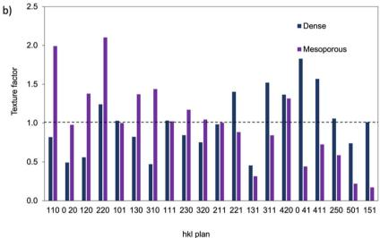
Fig. 12 (a) Relative intensity and (b) texture coefficients for different (hkl) planes of glass/FTO/c-TiO<sub>2</sub>/Sb<sub>2</sub>S<sub>3</sub> (dark blue) and glass/FTO/c-TiO<sub>2</sub>/ mp-TiO<sub>2</sub>/Sb<sub>2</sub>S<sub>3</sub> (purple) samples.
