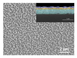
Fig. 9 SEM micrographs in top-view and cross-section (inset) of glass/FTO/c-TiO $_2$ /mp-TiO $_2$ /Sb $_2$ S $_3$  sample. The following color code is used to label the consecutive layers: FTO glass (turquoise), c-TiO $_2$  and mp-TiO $_2$  (yellow) infiltrated by Sb $_2$ S $_3$ , and overlayer of Sb $_2$ S $_3$  (purple).
