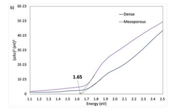
$\textbf{Fig. 13} \quad \textbf{(a) Absorbance spectra and (b) Tauc plots of glass/FTO/c-TiO_2/Sb_2S_3 (dark blue) and glass/FTO/c-TiO_2/mp-TiO_2/Sb_2S_3 (purple) samples. } \\$
