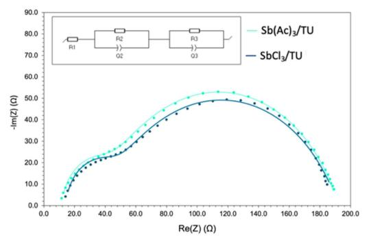
Fig. 7 EIS Nyquist plots of Sb(Ac)<sub>3</sub>/TU (turquoise) and SbCl<sub>3</sub>/TU (dark blue) Sb<sub>2</sub>S<sub>3</sub>-based solar cells; inset: the equivalent electrical circuit used for data fitting.
