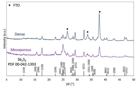
Fig. 11 X-ray diffractograms of glass-FTO/c-TiO<sub>2</sub>/Sb<sub>2</sub>S<sub>3</sub> (dark blue) and glass-FTO/c-TiO<sub>2</sub>/mp-TiO<sub>2</sub>/Sb<sub>2</sub>S<sub>3</sub> (purple) samples.
