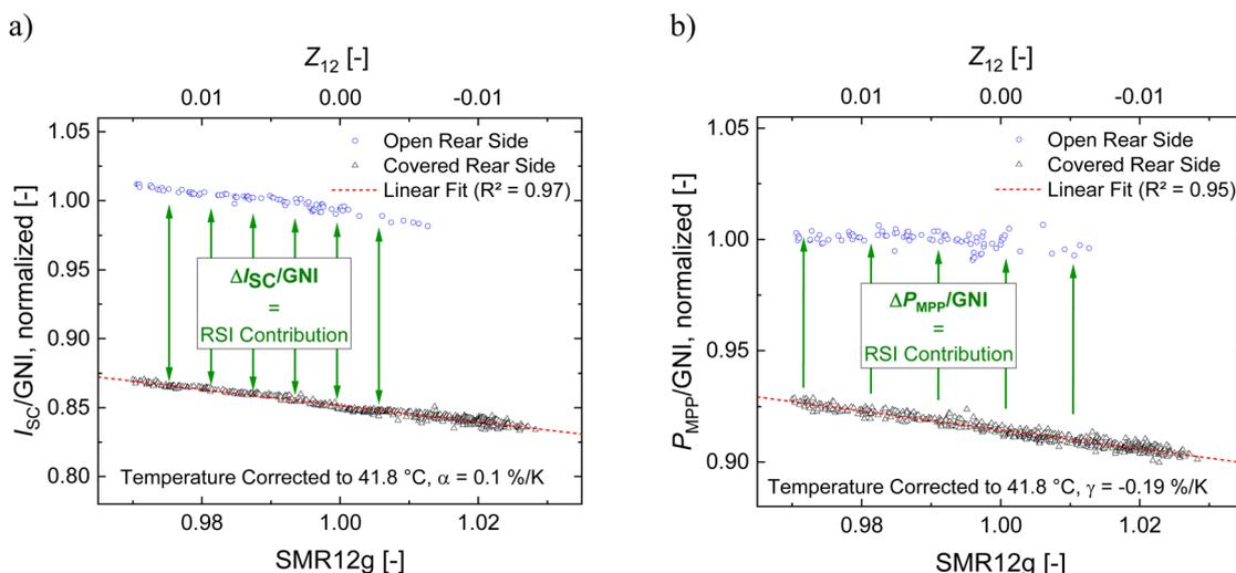
Fig. 6 (a) Calculation of the module's  $\sigma_{I_{SC}}$  based on a comparison of measurements carried out with an open (blue circles) and covered (black triangles) rear side of the module. All datapoints are temperature corrected to 41.8 °C, which was the mean operation temperature (standard deviation: 1.3 °C) of the module at reference spectral conditions. (b) Calculation of the modules  $\sigma_{P_{MPP}}$  analogous to the procedure in graph (a).
