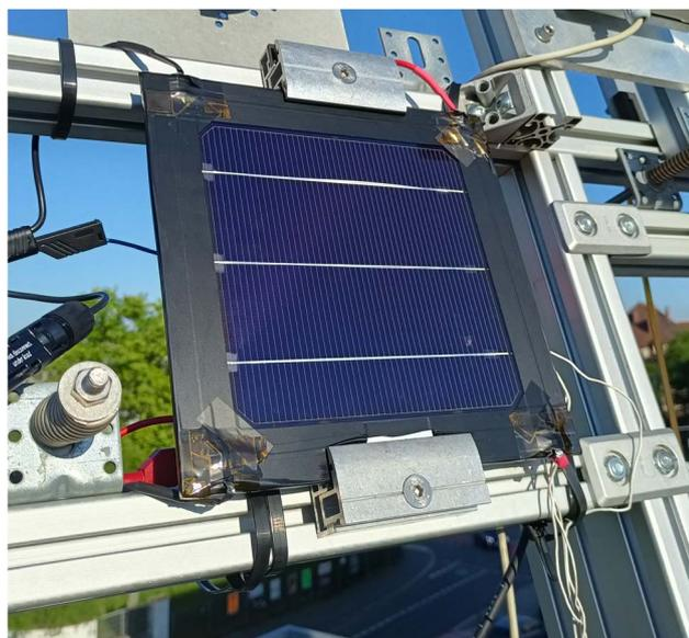
Fig. 1 PSC/Si single-cell module mounted on a dual axis tracker at our outdoor measurement setup in Freiburg, Germany, 48.01° N, 7.83° E.
