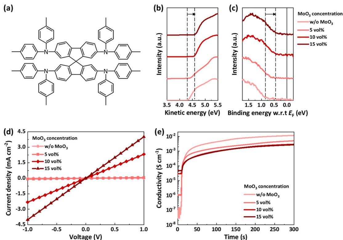
Fig. 1 (a) Molecular structure of spiro-TTB; (b) and (c) UPS spectra of (b) the secondary electron cut-off region and (c) the HOMO region; (d) J-V curves of the spiro-TTB:MoO<sub>3</sub> composite films with different MoO<sub>3</sub> concentrations; and (e) conductivity-time characteristics obtained from the spiro-TTB:MoO<sub>3</sub> composite films in an iodine-rich environment.
