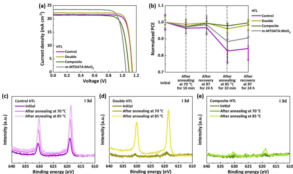
Fig. 2 (a)  $J$ - $V$  characteristics of PSCs incorporating different HTLs. The data for the  $m$ -MTDATA:MoO<sub>3</sub> HTL are from an earlier study.<sup>15</sup> (b) Normalized PCE measured at different aging conditions, and (c–e) I 3d XPS spectra of Au electrodes peeled off from PSCs with different HTLs.
