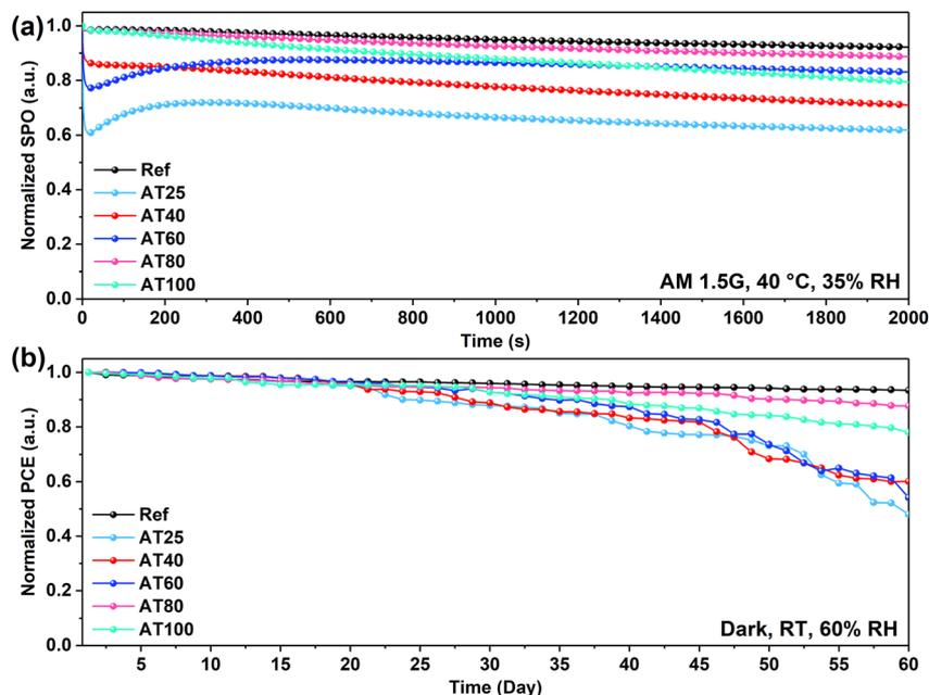
**Fig. 6** Long-term device stability (a) under AM1.5G solar irradiation, 40 °C, and 35% RH, and (b) under dark conditions, room temperature, and 60% RH, for champion PSCs based on perovskite films annealed at different temperatures in the ASB approach.
