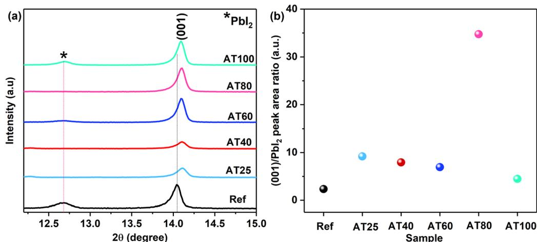
Fig. 3 (a) The magnified XRD pattern for reference sample and 3-hal perovskite films grown on ITO/compact-SnO<sub>2</sub> substrates with different annealing temperatures, and (b) (001) to PbI<sub>2</sub> peak area ratio at different annealing temperatures.
