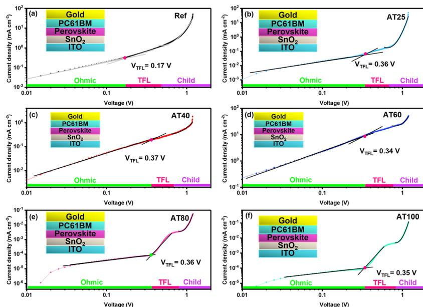
Fig. 8 The  $J$ - $V$  graphs of (ITO/compact-SnO<sub>2</sub>/perovskite/PC61BM/Au) devices for the (a) reference device and with different annealing temperatures of (b) 25, (c) 40, (d) 60, (e) 80, and (f) 100 °C, with the electron-only structure shown in the inset.
