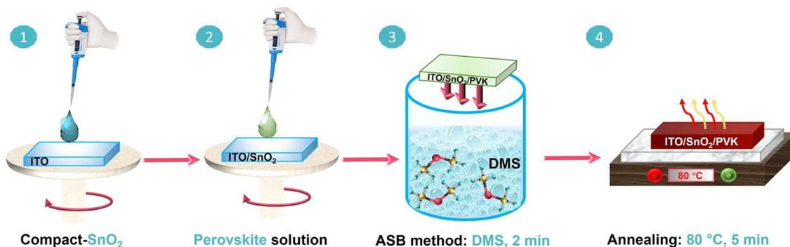
**Fig. 1** Sequential schematic of perovskite film fabrication using an ASB approach, Step 1: deposition of compact SnO<sub>2</sub> layer on ITO coated glass substrate, step 2: spin coating of mixed cation–anion perovskite solution on ITO/SnO<sub>2</sub>, step 3: submerging the substrate in the DMS bath as antisolvent for 2 min, step 4: crystallization of perovskite film by annealing at optimized temperature of 80 °C, for 5 min.
