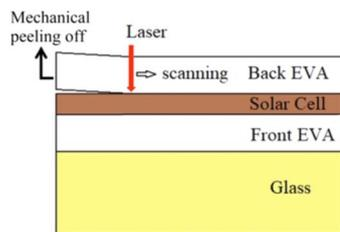
Fig. 5 Working process for the back EVA recycling via the laser irradiation followed by mechanical peeling method.<sup>72</sup> Elsevier, Copyright 2021.
