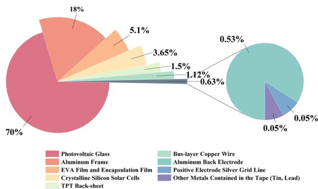
Fig. 3 The mass percentage of each component in a typical crystalline silicon photovoltaic module.<sup>8</sup>
