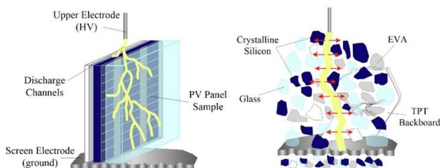
Fig. 9 Schematic diagram of high-pressure pulse crushing,<sup>90</sup> Elsevier, Copyright 2020.
