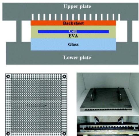
Fig. 6 Schematic diagram of mechanical fixture,<sup>71</sup> RSC, Copyright 2016.
