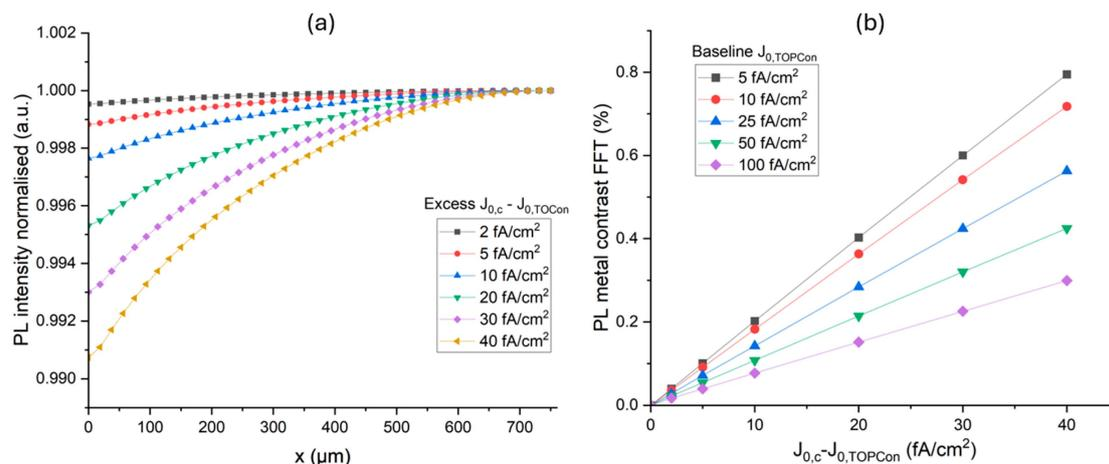
Fig. 5 (a) Normalised PL intensity line profile series in the unit cell, with a  $J_{0,\text{TOPCon}} = 10 \text{ fA cm}^{-2}$ , and varying excess  $J_{0,c} - J_{0,\text{TOPCon}}$  (b) PL metal contrasts extracted by FFT vs. excess  $J_{0,c} - J_{0,\text{TOPCon}}$ .
