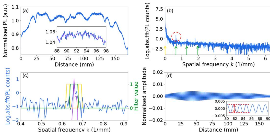
Fig. 3 (a) Original PL counts in  $x$ -domain along a line profile in the horizontal image direction, with inset showing noised-covered periodicity. (b) FFT-transformed line profile in  $k$ -domain. (c) A zoom-in in  $k$ -domain towards the peak at fundamental metal line frequency, with filter windows displayed as overlays. (d) Reconstructed signal and with inset showing wave amplitude.
