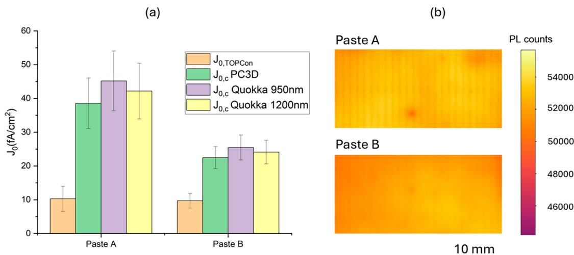
Fig. 6 (a) Estimated baseline  $J_{0,\text{TOPCon}}$  values, and  $J_{0,c}$  values extracted using both PC3D and Quokka for metal paste A and B. (b) PL image examples from a paste A sample a paste B sample, on same colour scale, enlarged to demonstrate the difference in metal line contrast.
