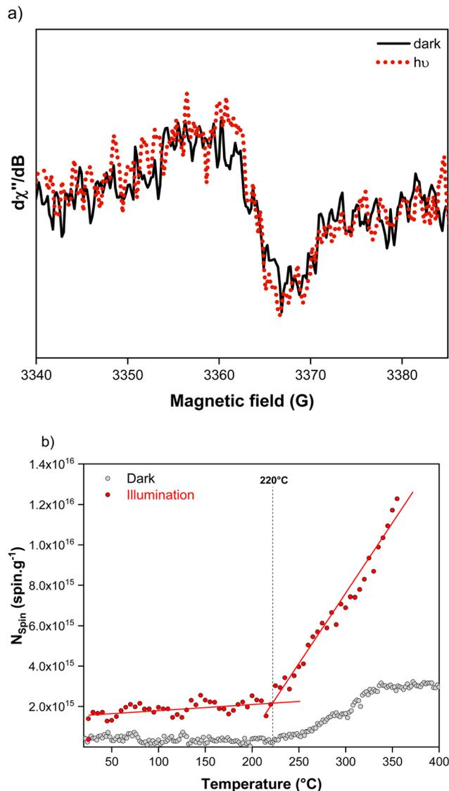
Fig. 3 (a) Comparison of EPR spectra of (FA-MA)PbI<sub>3</sub> in the dark (black line) and under illumination (red dashes) at 25 °C. (b) Comparison of the evolution of the spin density of (FA-MA)PbI<sub>3</sub> as a function of temperature in the dark (black) and under illumination (red). For illumination measurements, the lamp was turned on *ca.* 1 minute before starting the EPR acquisition.
