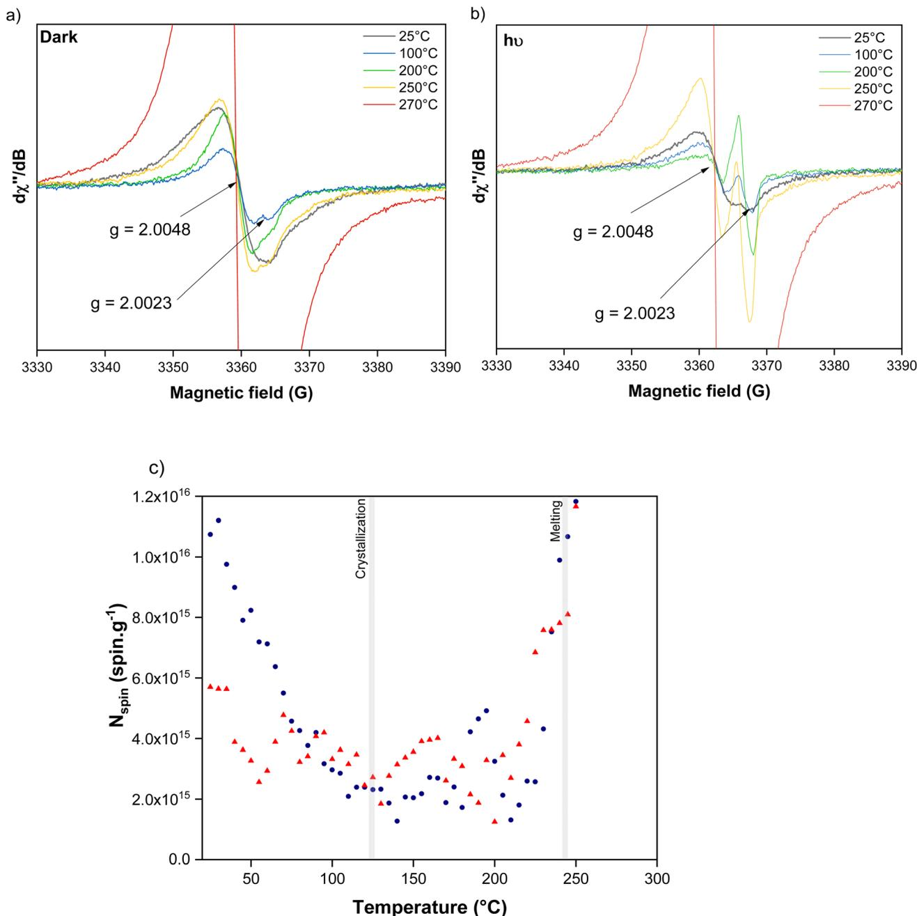
Fig. 4 Electron paramagnetic resonance spectroscopy on (FA-MA)PbI<sub>3</sub>/spiro-OMeTAD as a function of temperature between 20 °C and 300 °C: (a) in the dark, (b) under illumination, (c) comparison of the evolution of spin concentration as a function of temperature in the dark (blue) and under illumination (red). For illumination measurements, the lamp was turned on *ca.* 1 minute before starting the EPR acquisition.
