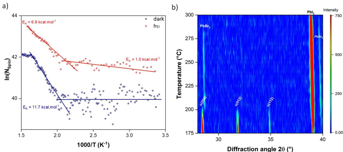
Fig. 2 (a) Arrhenius plot of spin concentration depending on temperature for the perovskite in the dark (blue) and under illumination (red) with the corresponding activation energies  $E_A$ . (b) 2D contour plot representation of *in situ* X-ray diffraction at temperatures between 175 °C and 300 °C for (FA-MA)PbI<sub>3</sub> film.
