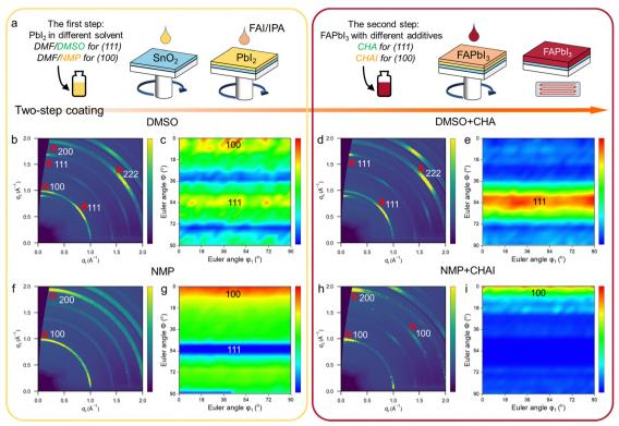
Fig. 1 (a) Schematic representation of the fabrication method for the solvent-additive cascade regulation (SACR) strategy. (b), (d), (f) and (h) GIWAXS and (c), (e), (q) and (i) ODF results of perovskite films prepared with different solvent systems without or with the SACR method.
