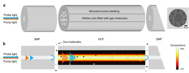
Fig. 1 The HCF-PTS gas sensor. (a) Schematic of the HCF gas sensor with the cross-sectional image provided on the righthand side. (b) The temperature (hence RI) profile over the HCF. The intensity profiles of the probe and pump beams and gas molecules are also superimposed onto the temperature profile. The angled end-face of the SMF eliminates the parasitic reflection.
