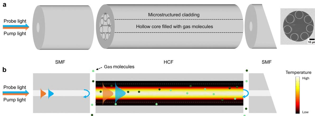
**Fig. 1** The HCF-PTS gas sensor. (a) Schematic of the HCF gas sensor with the cross-sectional image provided on the righthand side. (b) The temperature (hence RI) profile over the HCF. The intensity profiles of the probe and pump beams and gas molecules are also superimposed onto the temperature profile. The angled end-face of the SMF eliminates the parasitic reflection.
