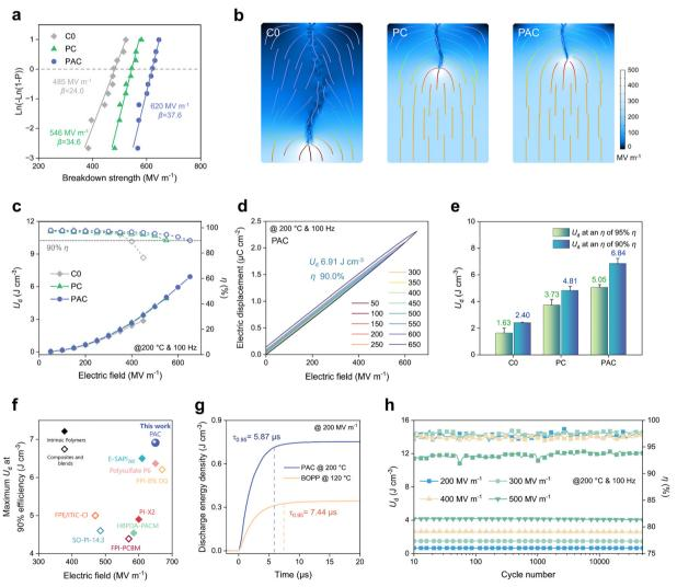
Fig. 4 Capacitive performances and stability of polymers. (a) Breakdown strengths and (b) electrical tree propagation simulations of CO, PC and PAC. (c) Capacitive performances of polymers at 200  $^{\circ}$ C & 100 Hz. (d) P-E loops of PAC. (e) Average maximum  $U_d$  at high efficiency of polymers. (f) Comparison of the energy storage performance at 200 °C and 90% efficiency. (g) Rapid discharge tests, with the load resistance ( $R_1$ ) of 100 k $\Omega$ . (h) Cycling stability of PAC.
