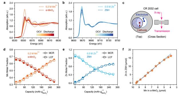
Fig. 2 Operando XANES at the Mn (a) and Zn (b) K-edge on  $\alpha$ -MnO<sub>2</sub> cathode. The LCF fitting and statistical MCR-ALS results were compared for both the Mn (d) and Zn (e) K-edges. Sketch of the experimental geometry used to acquire operando XAS (c). Correlation of absolute Zn and Mn amounts in the cell based on the edge jump of operando XAS (f).
