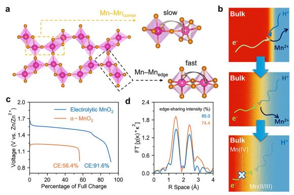
Fig. 5 Proposed mechanism for the evolution of the  $\alpha$ -MnO<sub>2</sub> surface during discharge (a), scheme for the charge transfer required in the second step of MnO<sub>2</sub> dissolution (b), and comparison of discharges for obtained by two different MnO<sub>2</sub> phases with respect to the theoretical capacity. (c) and the respective FTs-EXAFS (d).
