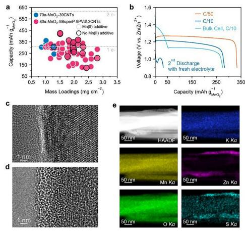
Fig. 1 First discharge capacities obtained from several cells using cathodes of different conductivities and mass loadings, with and without the MnSO<sub>4</sub> additive (a). Additional attempts to enhance the capacity of  $\alpha$ -MnO<sub>2</sub> with low C rate (C/50), excess electrolyte (bulk cell), and refreshing electrolyte (C/10) (b). STEM-HAADF images of pristine (c), and the discharged (d) electrodes. TEM-EDX maps of K, Mn, Zn, S, and O elements in the discharged sample (e).
