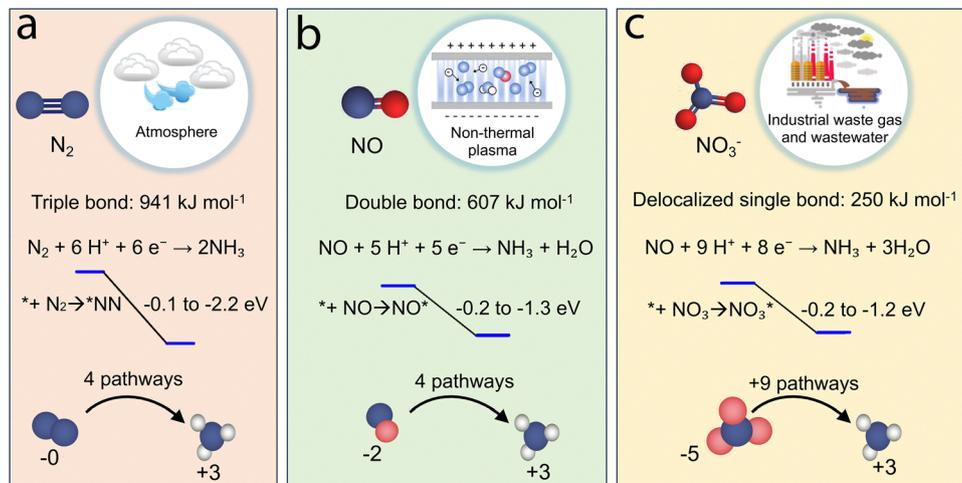
Fig. 2 Electroreduction pathways for ammonia synthesis from nitrogen species at different oxidation states, (a)  $\text{N}_2$  (0), (b)  $\text{NO}$  (+2), and (c)  $\text{NO}_3^-$  (+5), along with their respective sources, bond dissociation energies ( $\text{kJ mol}^{-1}$ ), overall reduction stoichiometries, and first-step adsorption free energies. Sphere colours denote nitrogen (blue), oxygen (red), and hydrogen (white).
