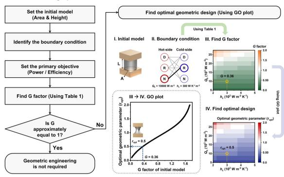
Fig. 2 Geometric design principle of a TE leg. Systematic flowchart illustrating the overall design process.
