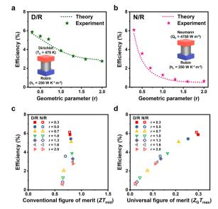
Fig. 4 Universal figure of merit incorporating geometric effects. (a) and (b)  $\eta_{\text{max}}$  as a function of r under (a) the Dirichlet-Robin boundary system and (b) the Neumann-Robin boundary system for seven different geometries (r = 0.3-2). (c) and (d) Plots of  $\eta_{\text{max}}$  versus (c) the conventional figure of merit ( $ZT_{mid}$ ) and (d) the universal figure of merit ( $Z_GT_{max}$ )
