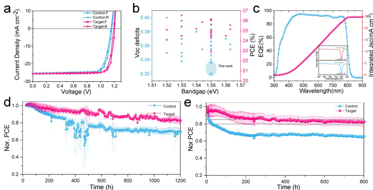
Fig. 4 (a)  $J$ - $V$  cure of the control, target PSCs. (b)  $V_{OC}$  and PCE statistics of devices with bandgaps close to approximately 1.55 eV. (c) EQE curves of champion-PSCs. Long-term operational stability under continuous output at MPP conditions (1 sun, LED lamps with ultraviolet filter); 65 °C (d) and 85 °C (e) in  $N_2$ -filled Chamber.
