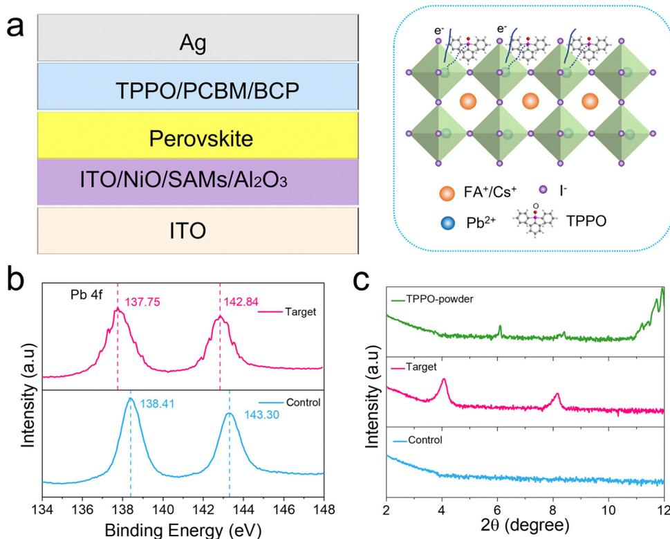
**Fig. 1** (a) The schematic diagram of interface modification in inverted perovskite solar cells via TPPO (left) and the chemical structure of TPPO molecule (right). (b) XPS spectra of Pb 4f (c) XRD patterns for control (PVK), target(w/TPPO), TPPO powder, a.u., arbitrary units.
