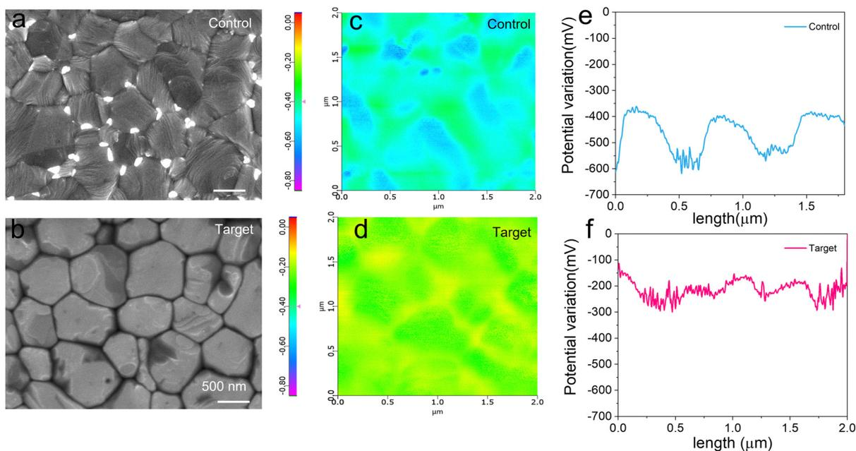
**Fig. 2** Top-view SEM images of the (a) control and (b) TPPO-treated perovskite films, Sample structure: ITO/NiOx/SAM/PVK (w, w/o TPPO). KPFM images of (c) the control and (d) TPPO-treated perovskite films. The corresponding line profiles (e) for the control film and TPPO-treated perovskite films (f). Sample structure: silicon wafer (Si)/NiOx/SAM/PVK (w, w/o TPPO).
