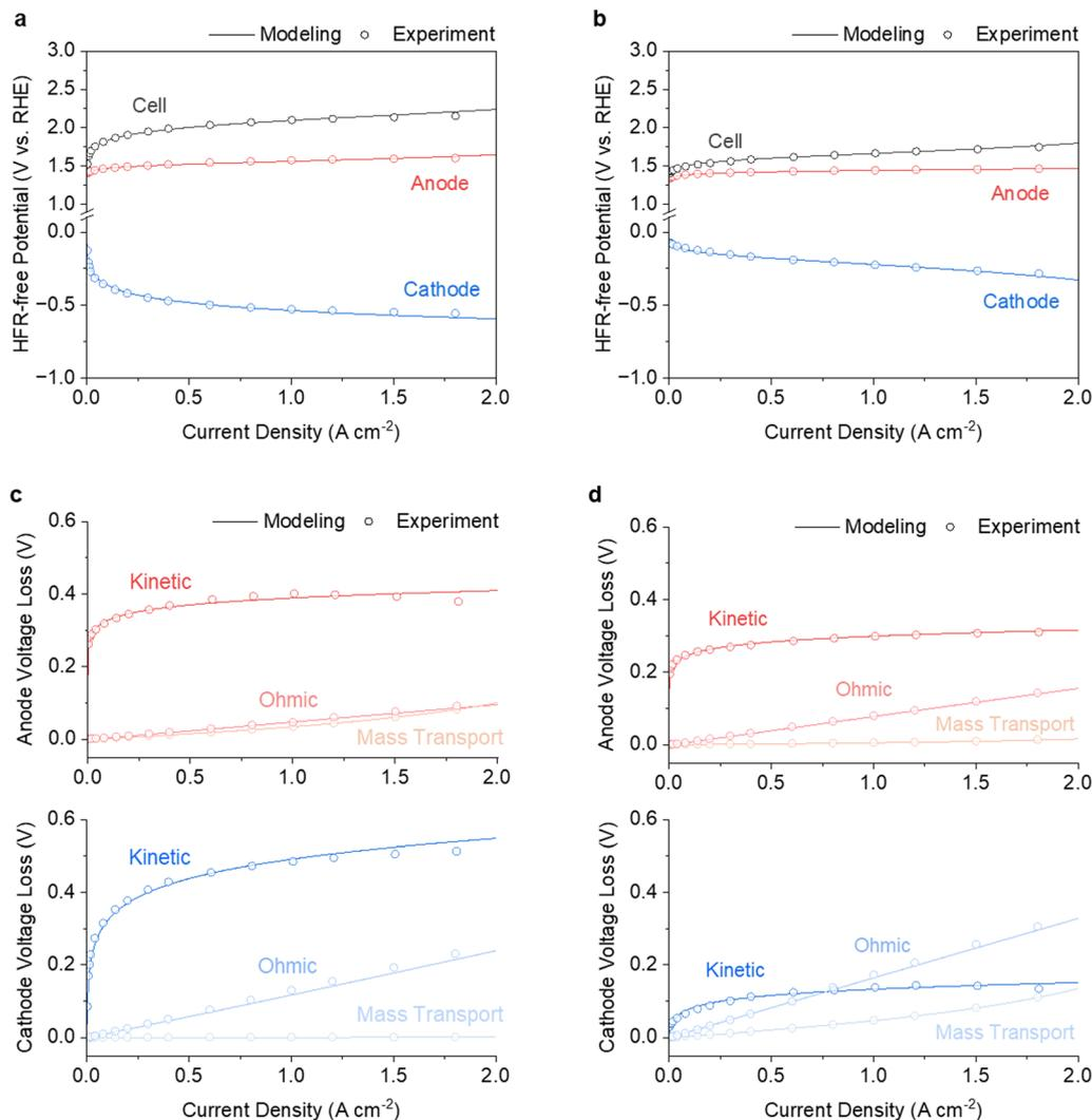
Fig. 3 Modeling analysis for each electrode and full cell at 1 atm and 80 °C. (a) and (b) Comparison of experimental (hollow circles) and modeled (solid lines) HFR-free polarization curves for the bare nickel foam reference (a) and Pt/C + NiFe (both) configuration (b). (c) and (d) Voltage breakdown results for the bare nickel foam reference (c) and Pt/C + NiFe (both) configuration (d), with anodic and cathodic contributions shown in the upper and lower panels, respectively.
