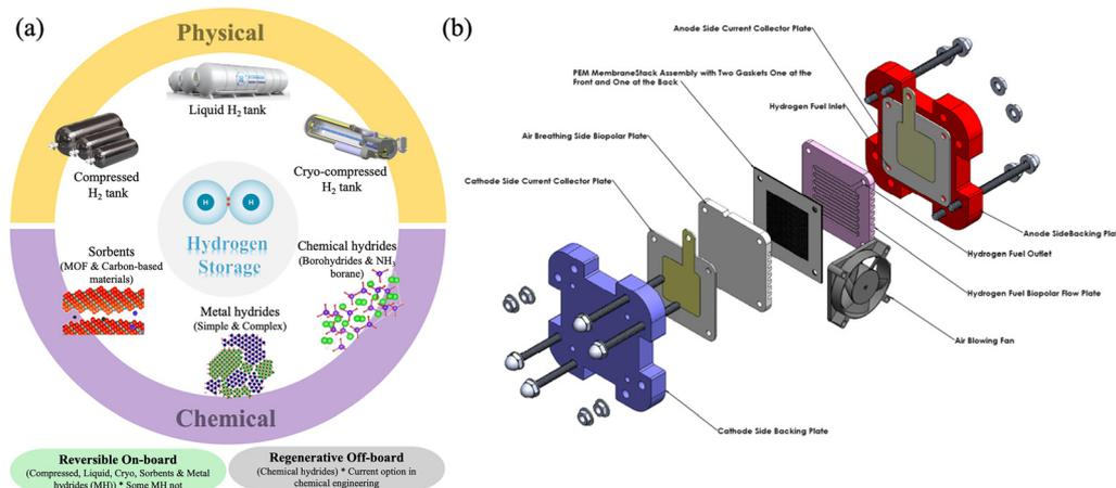
Fig. 5 (a) Classification of hydrogen-storage technologies. (b) Exploded view of a proton exchange membrane (PEM) fuel cell showing its key structural components. Adapted with from ref.<sup>75</sup> Copyright 2017, Elsevier.
