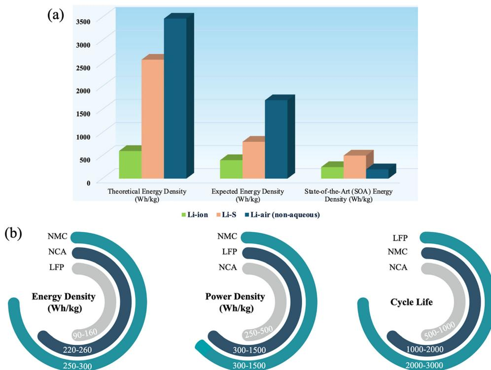
Fig. 7 (a) Comparison of the energy densities of potential battery chemistries for aviation applications, based on values from ref. 146–150. (b) Analysis of various lithium battery chemistries for aviation.
