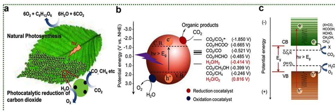
Fig. 28 (a) Schematic of artificial photosynthesis system. (b) Schematic illustration of the reaction mechanism. (c) Relative energy levels involved in semiconductor photocatalytic  $CO_2$  reduction. Reproduced from ref. 243 with permission from American Chemical Society, copyright 2017.
