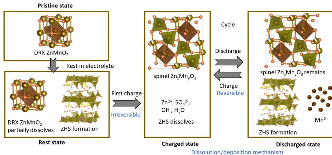
Fig. 5 Schematic of the energy storage mechanism for the ZnMnO<sub>2</sub> DRX cathode in an aqueous ZIB.
