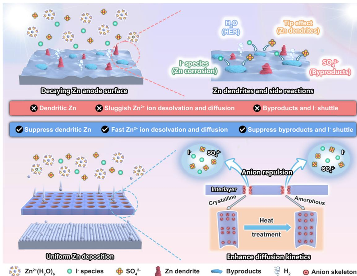
**Scheme 1** The role of the artificial interlayer based on the anion skeleton in inhibiting Zn dendrite and other side reactions on the Zn anode and its amorphous transformation in enhancing ion diffusion kinetics.
