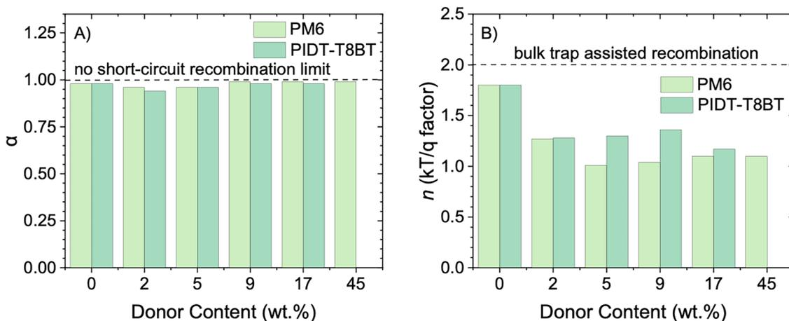
Fig. 5 Electrical characterization of L8BO devices with varying donor content reveal that trap-assisted recombination is dominant for low donor devices. (A) Variation of the slope of  $J_{sc}$  vs.  $\ln(I)$ . (B) Variation of ideality factor  $n$ , determined from the slope of  $V_{oc}$  vs.  $\ln(I)$ .
