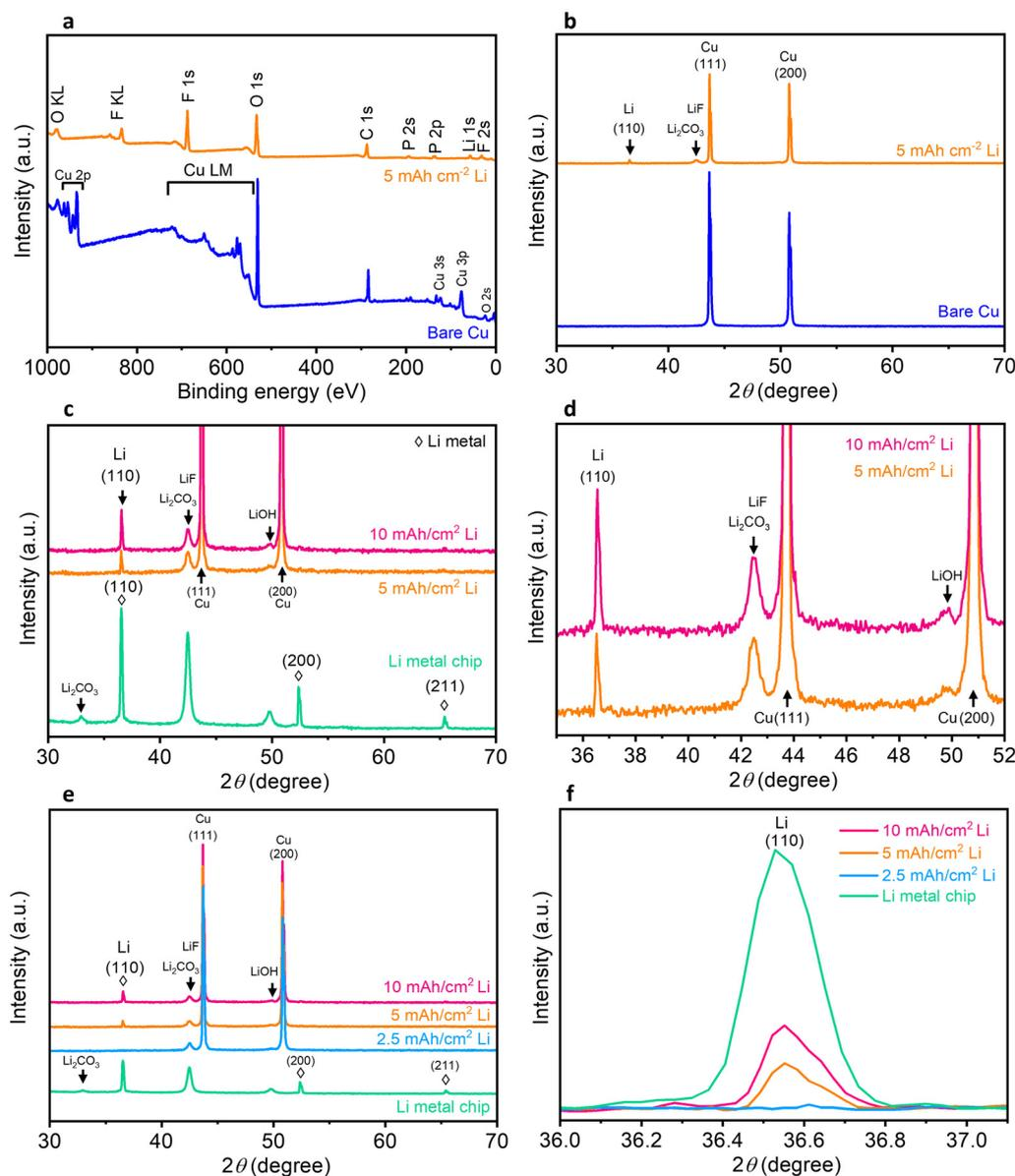
Fig. 2 (a) XPS survey spectra and (b) XRD patterns of the 5 mA h cm<sup>-2</sup> plated initial lithium and bare Cu-CC. (c) XRD patterns of a lithium metal chip, 5 and 10 mA h cm<sup>-2</sup> lithium metal plating, along with their magnified patterns (d). (e) XRD patterns of a lithium metal chip, 2.5, 5, and 10 mA h cm<sup>-2</sup> lithium metal plating, as well as their magnified Li (110) peak patterns (f).
