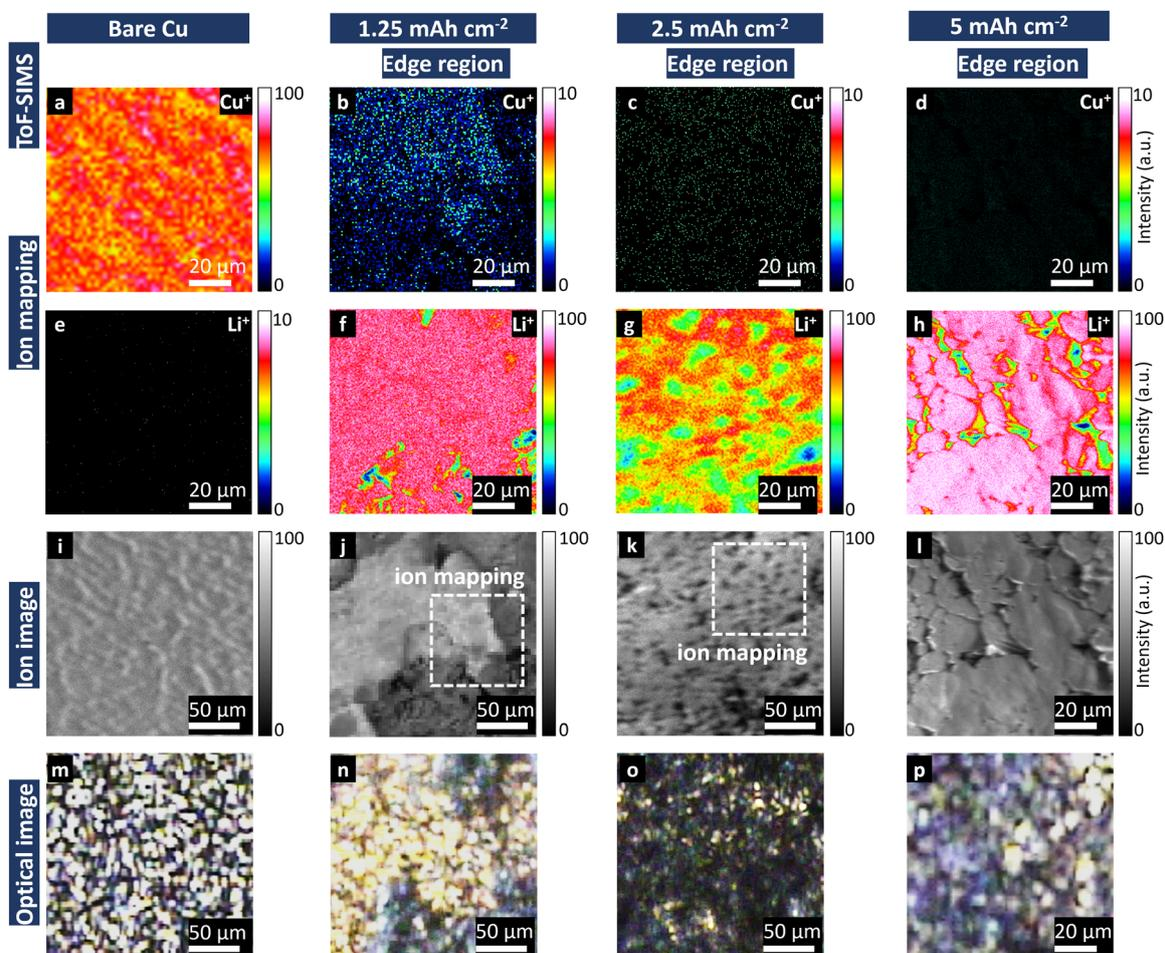
Fig. 5 (a)–(l) ToF-SIMS mapping and (m)–(p) optical images of the bare Cu-CC surface and annular edge regions of lithium metal plating with various capacities. The specific regions of  $\text{Cu}^+$  and  $\text{Li}^+$  ion mapping were marked within the larger-scale total ion images (j) and (k).
