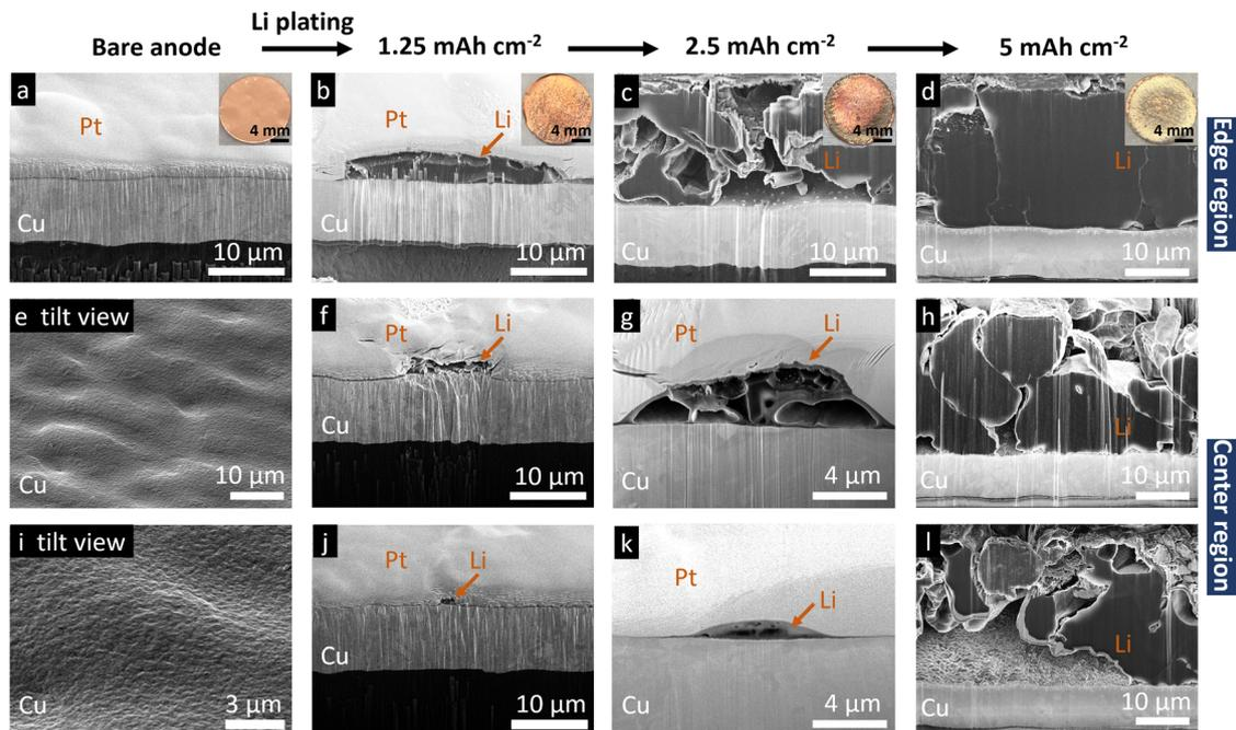
Fig. 4 (a)–(l) PFIB cross-section SEM images of the bare Cu-CC surface at different scales and the annular edge and center regions of various capacities lithium metal plating.
