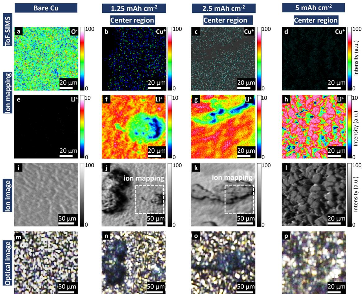
Fig. 6 (a)–(l) ToF-SIMS mapping and (m)–(p) optical images of the bare Cu-CC surface and center regions of various capacities lithium metal plating. The specific regions of  $\text{Cu}^+$  and  $\text{Li}^+$  ion mapping were marked within the larger-scale total ion images (j), (k).
