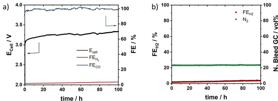
Fig. 5 Optimized stability test. (a) Cell voltage and FE of a stability test at  $100 \text{ mA cm}^{-2}$  using a  $1 \text{ M CsOH}$ . (b)  $\text{FE}_{\text{H}_2}$  and  $\text{N}_2$  vol% in the GC to prove no salt blocking. The data shown in the figure correspond to single tests.
