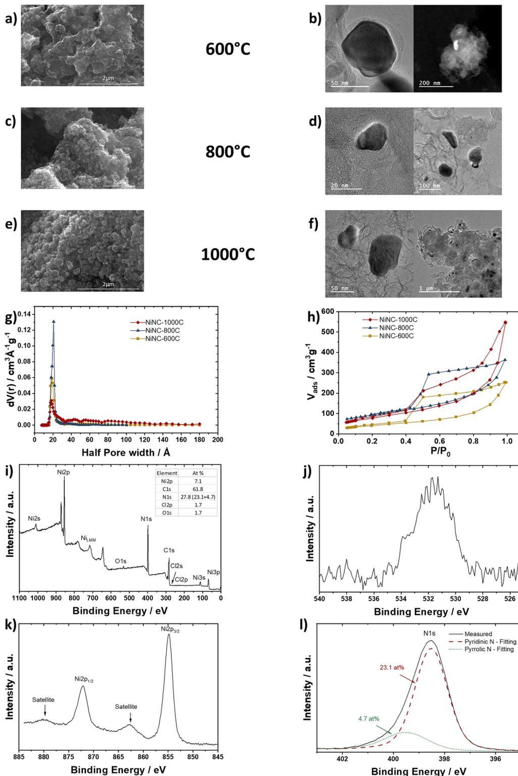
**Fig. 1** Characterization of the NiNC catalyst. (a) SEM and (b) TEM images of the NiNC-600C. (c) SEM and (d) TEM images of the NiNC-800C. (e) SEM and (f) TEM images of the NiNC-1000C. (g) Pore distribution and (h) adsorption/desorption isotherm plots. (i) survey XPS of NiNC-1000C, (j) insights of satellite and main peaks of nickel, (k) oxygen and (l) nitrogen, respectively.
