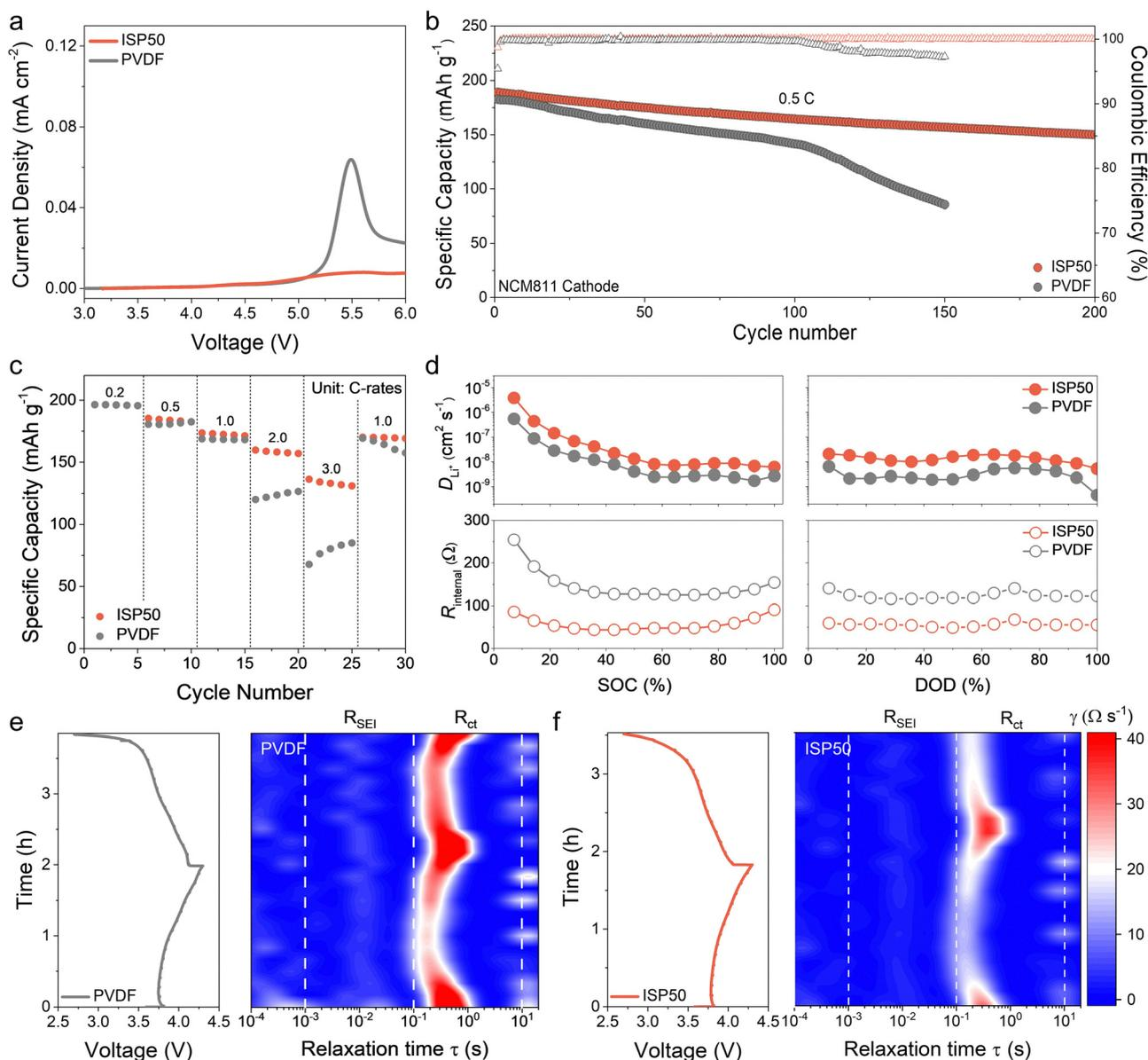
Fig. 4 (a) Linear sweep voltammetry (LSV) results from different binders. (b) Long-term cycling performance and (c) discharge rate capability NCM811 cathodes. (d) Internal resistance and  $\text{Li}^+$  diffusion coefficient of the Li||NCM811 cells as a function of SOC and DOD. *In situ* DRT results of a Li||NCM811 cell with (e) PVDF and (f) ISP50 binders.
