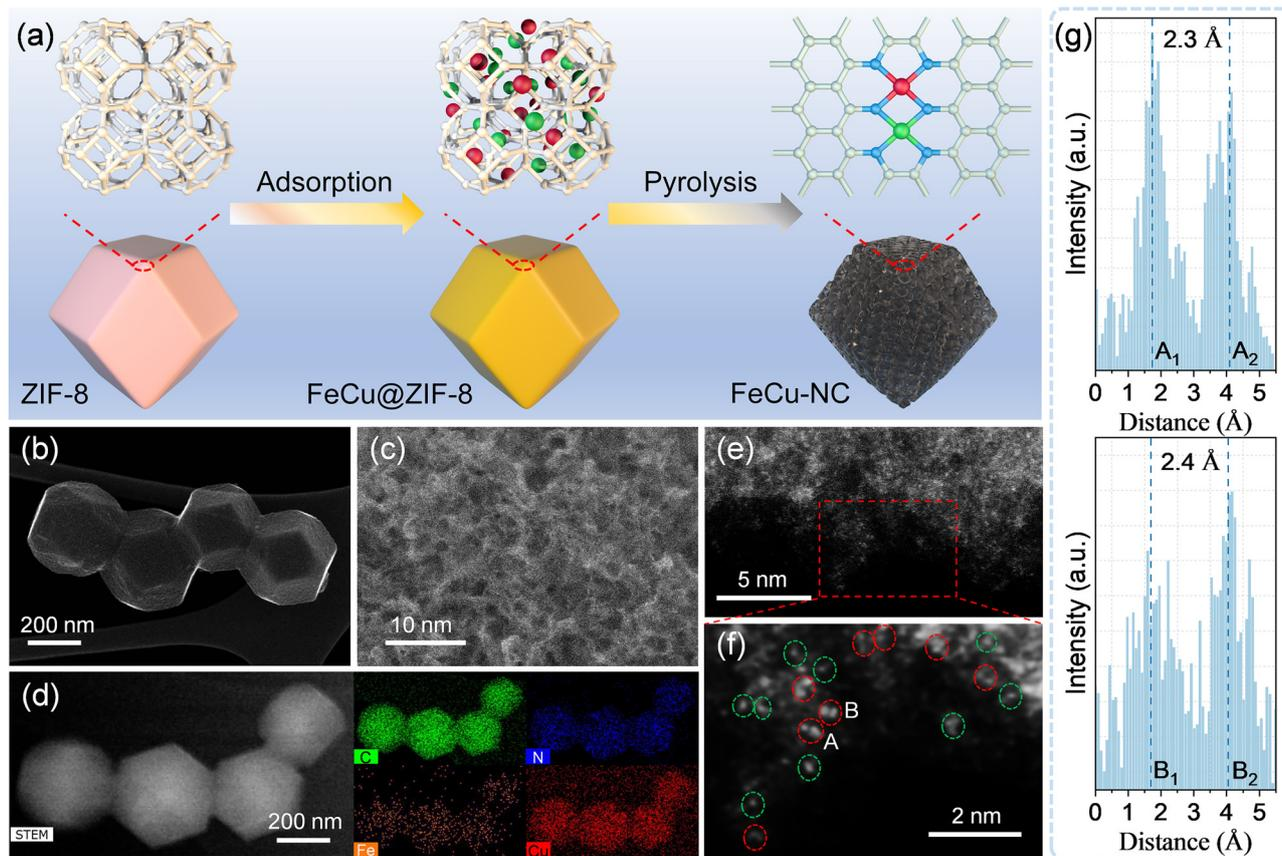
**Fig. 1** (a) Schematic illustration of the FeCu–NC synthesis process. (b) and (c) SEM images of FeCu–NC at different magnifications. (d) HAADF-STEM image and corresponding EDS element mapping of FeCu–NC. (e) and (f) Aberration-corrected HAADF-STEM images of FeCu–NC, with bimetallic pairs indicated by red circles and isolated metal atoms by green circles. (g) Intensity profiles obtained from two pairs in (f), labelled as A and B.
