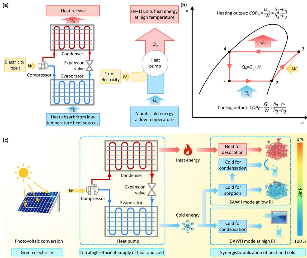
Fig. 3 The framework of next-generation solar-powered HAWH. (a) Working principle of a heat pump. (b) Diagram showing the thermodynamic cycle of the heat pump. 1-2: isobaric heat absorption, 2-3: isentropic compression, 3-4: isobaric heat release, 4-1: throttling. (c) Framework of the proposed solar-powered dual-mode HAWH by integrating DAWH and SAWH within a PV-powered heat pump, working under SAWH mode at low RH and DAWH mode at high RH.
