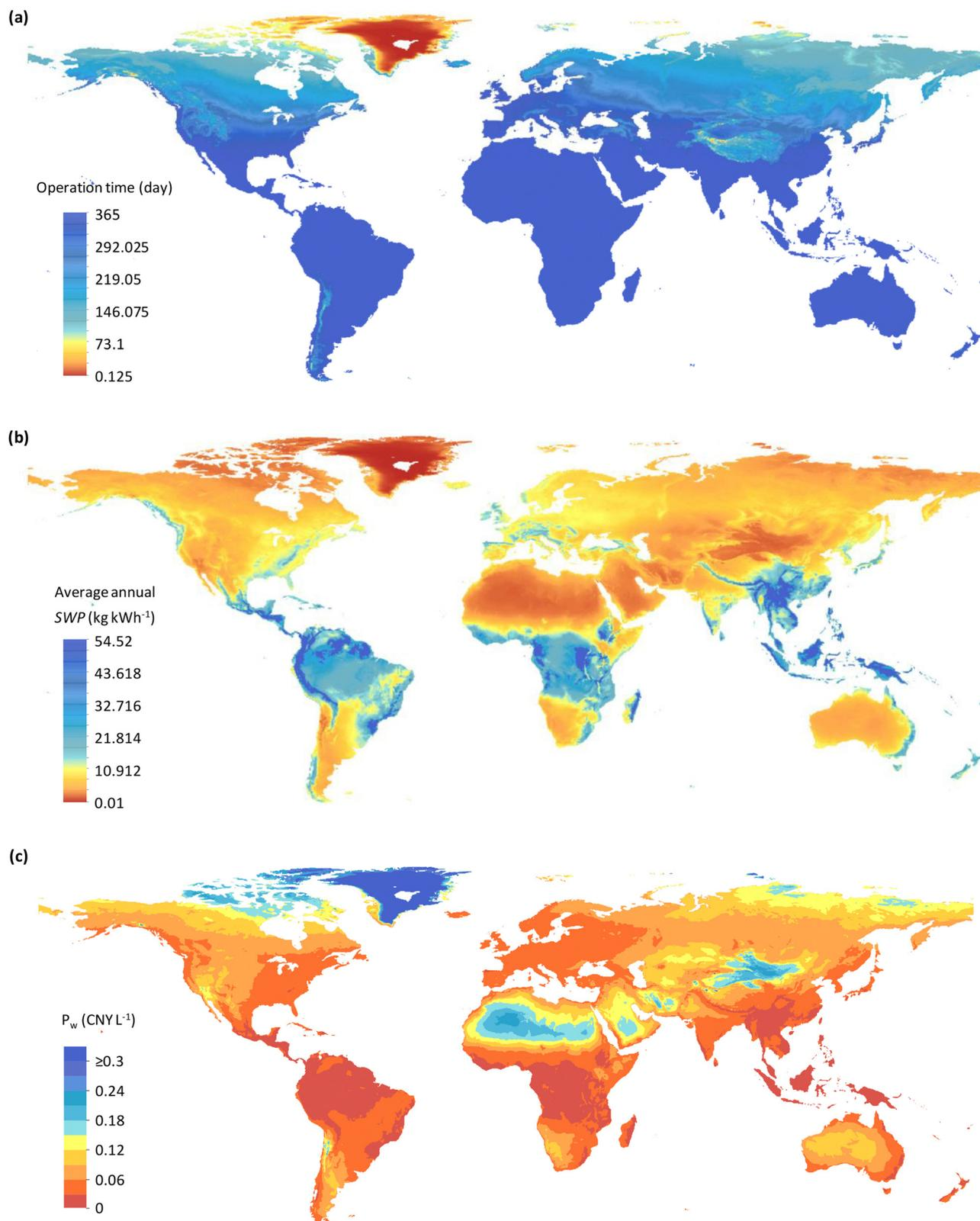
**Fig. 6** Climatic adaptability, energy-saving potential, and technoeconomic feasibility assessment of the HAWH under various global climates. (a) Year-round operation time of the HAWH. (b) Average annual specific water production of the HAWH. (c) The theoretical unit price of the produced water of the HAWH.
