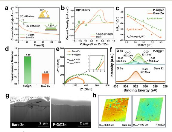
Fig. 3 Regulation of the Zn<sup>2+</sup> deposition behavior of the P-G SEI layer. (a) CA curves at -150 mV overpotential. (b) CV curves. (c) Arrhenius curves. (d)  $Zn^{2+}$  transference numbers of bare Zn and P-G@Zn symmetric cells. (e) Ionic conductivity (unit: mS cm<sup>-1</sup>). (f) XPS spectra of O 1s. (g) Cross-section SEM images of cycled anodes post FIB etching. (h) Surface roughness of cycled anodes after 30 cycles (1 mA cm<sup>-2</sup>, 1 mAh cm<sup>-2</sup>).
