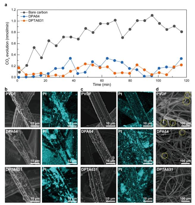
Fig. 5 Evaluation of carbon corrosion and catalyst detachment at the air electrode. (a) In situ DEMS analysis of the CO2 evolution quantification result. SEM and elemental mapping images (Pt) of air electrodes (b) before (c) after 100 charge/discharge cycles, and (d) SEM images showing carbon corrosion at the air electrode
