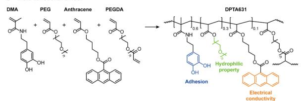
Fig. 1 Aqueous sodium-air batteries (Scheme). (a) air electrode assembled with a polymer binder, Pt catalyst, and carbon current collector in aqueous media, and (b) molecular design of a multi-functional binder with underwater adhesion and electrical conductivity
