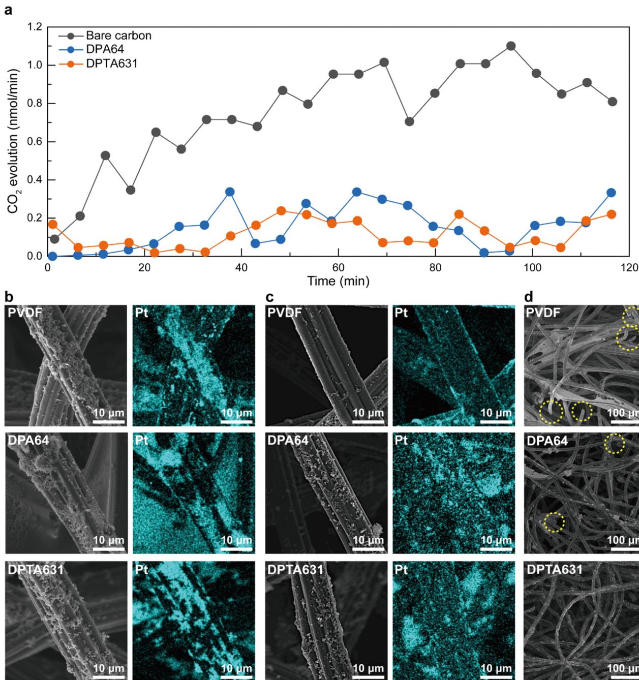
Fig. 5 Evaluation of carbon corrosion and catalyst detachment at the air electrode. (a) *In situ* DEMS analysis of the CO<sub>2</sub> evolution quantification result. SEM and elemental mapping images (Pt) of air electrodes (b) before (c) after 100 charge/discharge cycles, and (d) SEM images showing carbon corrosion at the air electrode.
