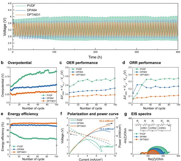
Fig. 2 Electrochemical performance of SABs. (a) Galvanostatic charge/discharge profiles, (b) overpotential, (c) OER and (d) ORR performance, (e) energy efficiency, (f) polarization curves and power densities, and (g) electrochemical impedance spectroscopy (EIS) spectra and equivalent circuit of SABs assembled with PVDF, DPA64 and DPTA631
