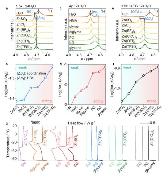
Fig. 2 Water-holding ability. (a)–(f) Evolution of  $^1H$  NMR spectra from  $H_2O$  (a), (c) and (e) and assessment of the water-holding ability via  $log(|\Delta\sigma_1|$  +  $|\Delta\sigma_2|$ ) (b), (d) and (f) in mixtures of 1.5x: 24H<sub>2</sub>O (a) and (b), 4y: 24H<sub>2</sub>O (c) and (d) and 1.5x: 4EG: 24H<sub>2</sub>O (e) and (f). x: salts. y: organics. (g) DSC curves of electrolytes with the composition of 1.5x:4y:24H<sub>2</sub>O during heating from -65 to 20 °C
