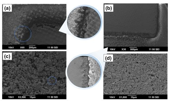
Fig. 3 SEM micrographs of (a) printed  $Ag_2Se$  and dielectric filler (brighter), (b) printed BST and dielectric filler (brighter), (c) n-type printed  $Ag_2Se$  leg, and (d) p-type printed BST leg.
