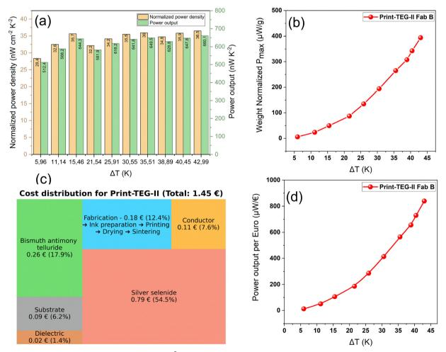
Fig. 9 (a) Normalized power density and power output/ $\Delta T^2$ . (b) Cost distribution for print-TEG II. (c) Fabrication cost distribution for print-TEG II. (d) Power output per Euro ( $\mu W$  per  $\epsilon$ ) at  $\Delta T$ s.
