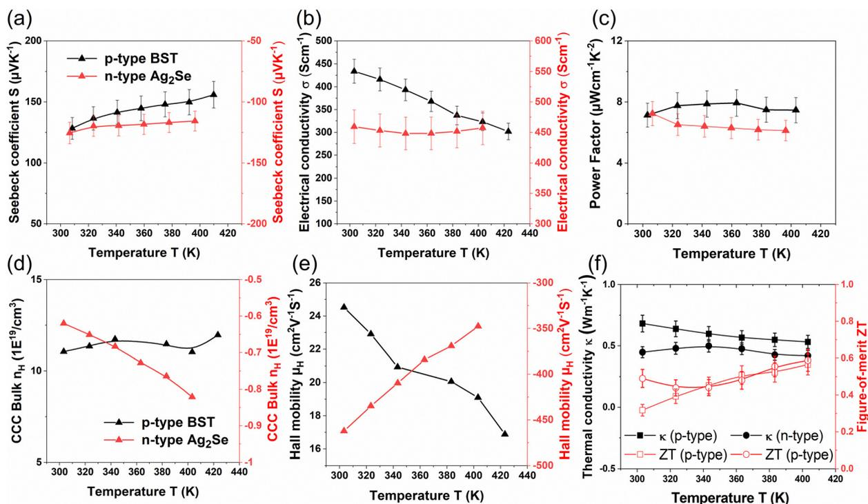
Fig. 4 Variation of the TE properties of p- and n-type legs vs. temperature. (a) Seebeck coefficient  $S$ , (b) electrical conductivity  $\sigma$ , (c) power factor  $S^2\sigma$ , (d) carrier concentration,  $n_H$  (e) Hall mobility  $\mu_H$ , and (f) thermal conductivity  $\kappa$  and figure-of-merit  $ZT$ .
