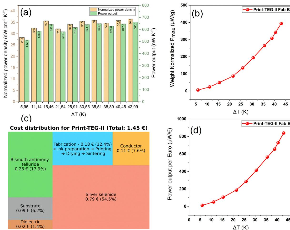
Fig. 9 (a) Normalized power density and power output/ $\Delta T^2$ . (b) Cost distribution for print-TEG II. (c) Fabrication cost distribution for print-TEG II. (d) Power output per Euro ( $\mu\text{W per } \text{€}$ ) at  $\Delta T$ s.
