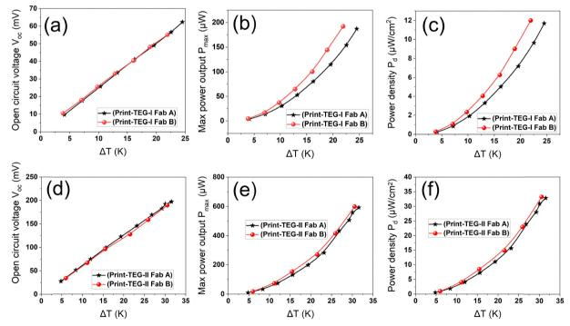
Fig. 8 Performance of print-TEG Fab A  $\theta$  Fab B. (a)  $V_{OC}$  of print-TEG I at  $\Delta T$ s. (b)  $P_{max}$  of print-TEG I at  $\Delta T$ s. (c)  $P_{d}$  of print-TEG I at  $\Delta T$ s. (d)  $V_{OC}$  of print-TEG II at  $\Delta T$ s. (e)  $P_{max}$  of print-TEG II at  $\Delta T$ s. (f)  $P_{d}$  of print-TEG II at  $\Delta T$ s.
