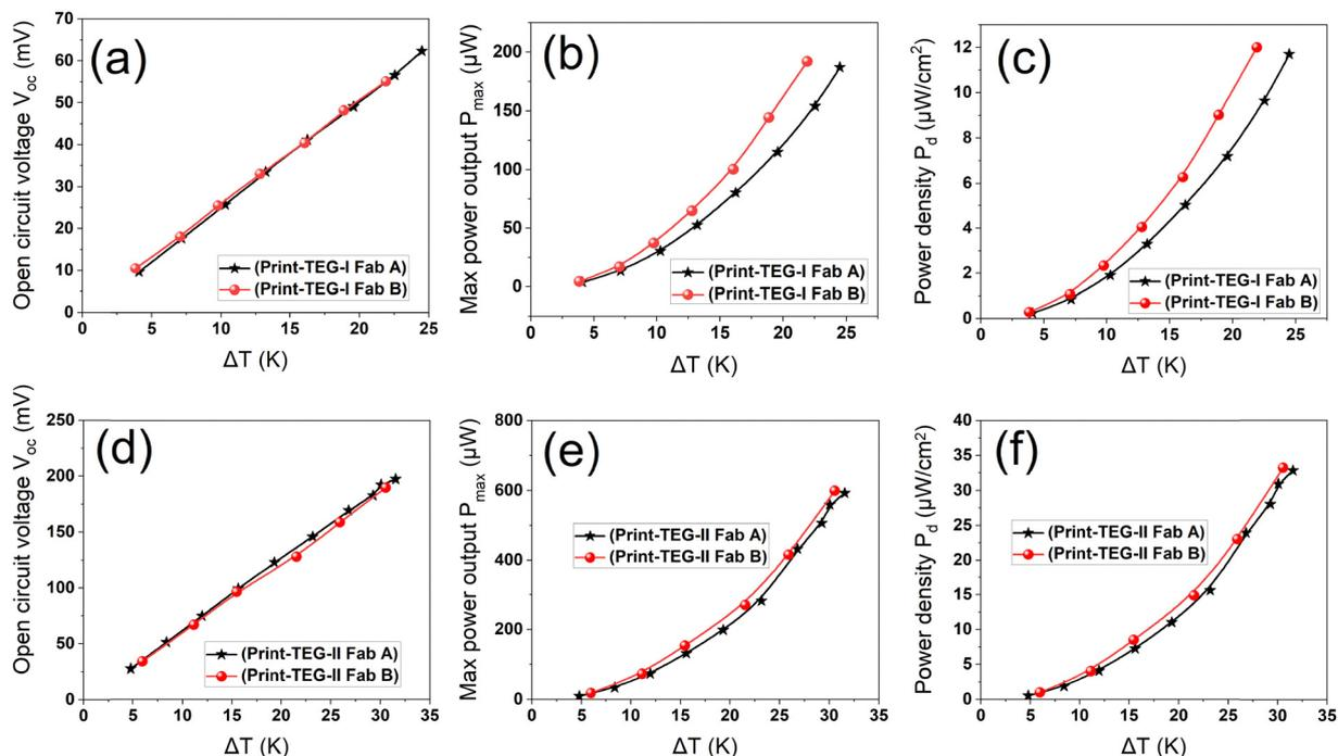
Fig. 8 Performance of print-TEGs Fab A & Fab B. (a)  $V_{OC}$  of print-TEG I at  $\Delta T$ s. (b)  $P_{max}$  of print-TEG I at  $\Delta T$ s. (c)  $P_d$  of print-TEG I at  $\Delta T$ s. (d)  $V_{OC}$  of print-TEG II at  $\Delta T$ s. (e)  $P_{max}$  of print-TEG II at  $\Delta T$ s. (f)  $P_d$  of print-TEG II at  $\Delta T$ s.
