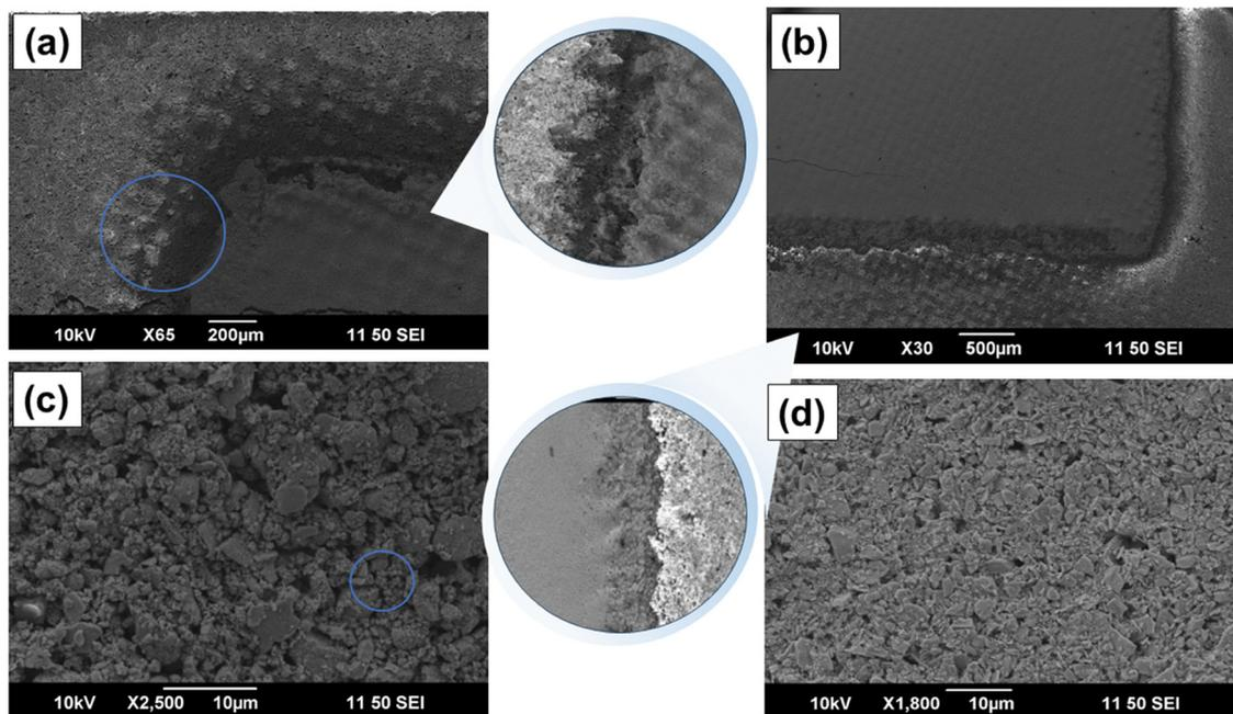
Fig. 3 SEM micrographs of (a) printed Ag<sub>2</sub>Se and dielectric filler (brighter), (b) printed BST and dielectric filler (brighter), (c) n-type printed Ag<sub>2</sub>Se leg, and (d) p-type printed BST leg.
