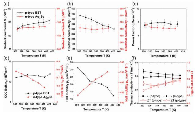
Fig. 4 Variation of the TE properties of p- and n-type legs vs. temperature. (a) Seebeck coefficient S, (b) electrical conductivity  $\sigma$ , (c) power factor  $S^2\sigma$ , (d) carrier concentration,  $n_{\rm H}$  (e) Hall mobility  $\mu_{\rm H}$ , and (f) thermal conductivity  $\kappa$  and figure-of-merit ZT.
