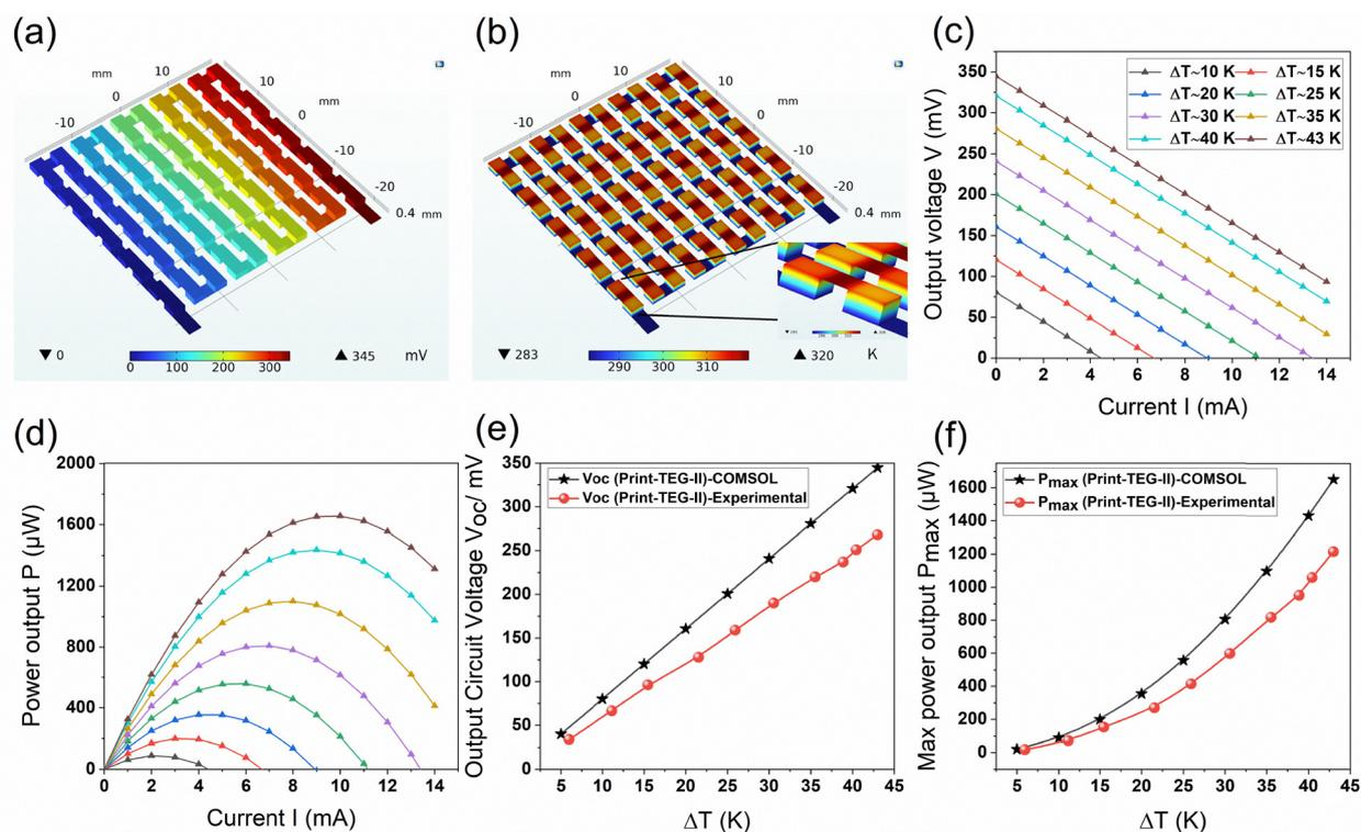
Fig. 7 COMSOL simulated model of print-TEG II. (a) Electric potential map of print-TEG II. (b) Thermal map of print-TEG II. (c) Simulated  $V-I$  characteristics at different temperatures. (d) Simulated  $P-I$  characteristics at different temperatures. (e) Comparison of open circuit voltage, simulated vs. experimental. (f) Comparison of Max power output, simulated vs. experimental.
