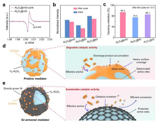
Fig. 3 Mechanism of active site failure and protection. (a) Ex situ EPR spectra of  $Al_2O_3$ @mG. (b) EPR intensity of different  $Al_2O_3$ @G samples before and after cycling. (c) Corresponding vacancy retention rates after 60 cycles at 1.0 C. Schematic illustrating the evolution of vacancy sites on (d) the pristine mediator and (e) the graphene-armored mediator during the electrochemical process.
