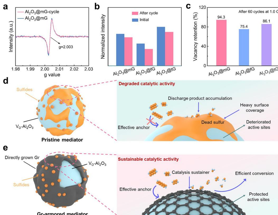
Fig. 3 Mechanism of active site failure and protection. (a) *Ex situ* EPR spectra of  $\text{Al}_2\text{O}_3@\text{mG}$ . (b) EPR intensity of different  $\text{Al}_2\text{O}_3@\text{G}$  samples before and after cycling. (c) Corresponding vacancy retention rates after 60 cycles at 1.0 C. Schematic illustrating the evolution of vacancy sites on (d) the pristine mediator and (e) the graphene-armed mediator during the electrochemical process.
