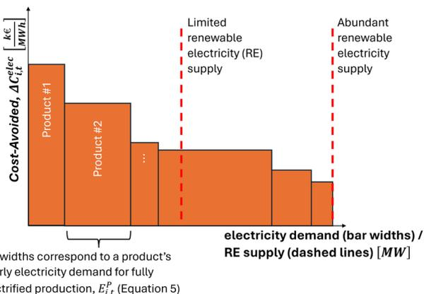
Fig. 2 Schematic representation of the time-dependent merit order curve arising from the *Cost-Avoided* of each product,  $\Delta C_{it}^{\text{elec}}$ , and their electricity demands,  $E_{it}^p$ . Here, for explanatory purposes, we show the intersection of two possible renewable electricity (RE) availabilities for a single merit order curve. However, a distinct merit order curve exists in each time step.
