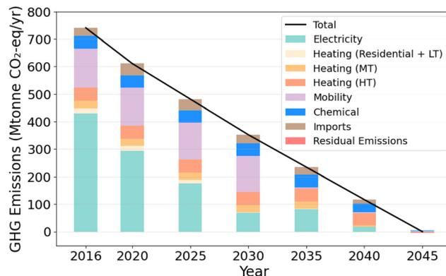
Fig. 3 GHG emissions, in million tonnes  $\text{CO}_2\text{-eq}$ , of the integrated energy system and chemical industry model by sector. The chemical industry transitions last along with medium temperature (MT) and high temperature (HT) heat starting in 2040. LT: low temperature.
