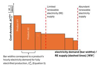
Fig. 2 Schematic representation of the time-dependent merit order curve arising from the Cost-Avoided of each product,  $\Delta C_{i,t}^{\text{elec}}$ , and their electricity demands,  $E_{i,t}^{P}$ . Here, for explanatory purposes, we show the intersection of two possible renewable electricity (RE) availabilities for a single merit order curve. However, a distinct merit order curve exists in each time step.
