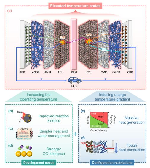
Fig. 1 Illustration of the reason for the MEA maintaining the elevated temperature states. (a) The fundamental operating principle of PEMFCs. (b) Enhanced reaction kinetics. (c) Simplified water and heat management. (d) Improved tolerance of the catalyst to CO impurities. (e) Massive heat generation within the MEA. (f) Low heat dissipation capability of the MEA components.
