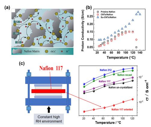
Fig. 6 (a) Schematic illustration of proton transportation in water-hydrated pristine Nafion membranes.<sup>111</sup> (b) Effect of operating temperatures on the proton conductivity. 111 (c) Proton conductivities of Nafion recast, Nafion 212, Nafion un-crystallized, and Nafion 117 as received and Nafion 117 oriented membranes as a function of temperature (20-120 °C) at 90% RH.<sup>15</sup>
