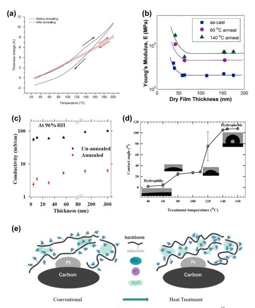
Fig. 12 (a) Thickness change of unannealed and annealed Nafion films (50 nm) on SiO<sub>2</sub> as a function of temperature.<sup>19</sup> (b) Young's modulus at 30% RH: as cast, 60 °C annealing, and 140 °C annealing, 24 (c) Proton conductivity of unannealed and annealed Nafion thin films at 96% RH and 60 °C. 158 (d) Surface wettability of annealed ultrathin (10 nm) Nafion film.<sup>136</sup> (e) Mechanism of enhanced local transport after heat treatment.<sup>137</sup>
