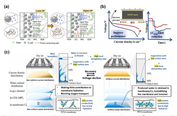
Fig. 20 (a) Schematic of operating pressure (OP) impacts on local mass transfer at higher loads: lower OP and higher OP.<sup>20</sup> (b) Schematic of the PEMFC performance improvement at elevated temperatures by increasing the inlet pressure.<sup>21</sup> (c) Schematic of the performance loss and recovery mechanism, where the 'undesirable' and 'desirable' water distributions are shown on the left and right respectively. 105
