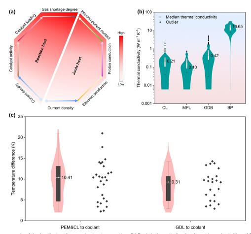
Fig. 2 (a) The influence rule of the key factors for massive heat generation. (b) Statistical results for the thermal conductivities of PEMFC components including the CL,  $^{23,38-52}$  microporous layer (MPL),  $^{23,38,40,42-47,49,51-54}$  gas diffusion backing (GDB),  $^{23,38,40,42-47,49,51,52,55-72}$  and bipolar plate (BP).  $^{23,38,40,42-47,49,51,52,73}$  (c) Statistical results for the temperature differences between the PEM and the CL, GDL and coolant.  $^{42,46,49,50,52,54,56,74-78}$
