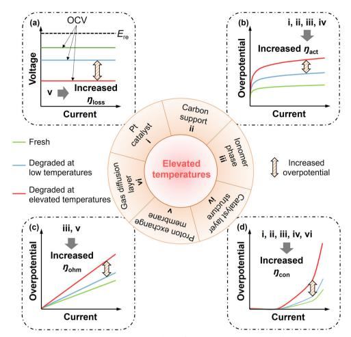
Fig. 18 Impacts of MEA component durability on performance loss of PEMFCs after the durability test at different temperatures
