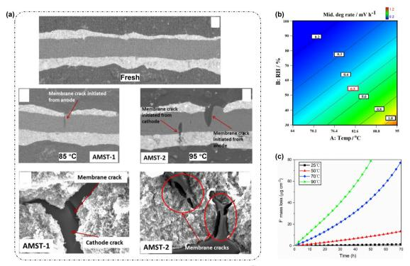
Fig. 15 (a) SEM images of fresh and degraded CCMs from the AMST-1 and AMST-2 tests.<sup>171</sup> (b) Contour plot of effects of temperature and humidity on the Mid. membrane degradation rate.<sup>207</sup> (c) Evolution of cumulative fluoride loss at different operating temperatures.<sup>184</sup>
