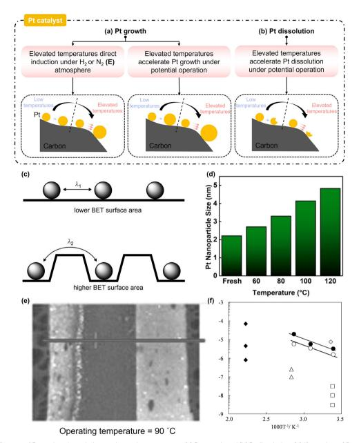
Fig. 9 Schemic diagram of Pt catalyst degradation at elevated temperatures: (a) Pt growth and (b) Pt dissolution. (c) Illustration of Pt particle growth as a function of the distance between the nanoparticles. 128 (d) Alterations in the Pt catalyst size as the cell temperature increases during voltage cycling (0.1-0.96 V).4 (e) Denser Pt microscopy images at the MEA cross-section. 125 (f) Logarithm of Pt solubility as a function of inverse temperature. 138
