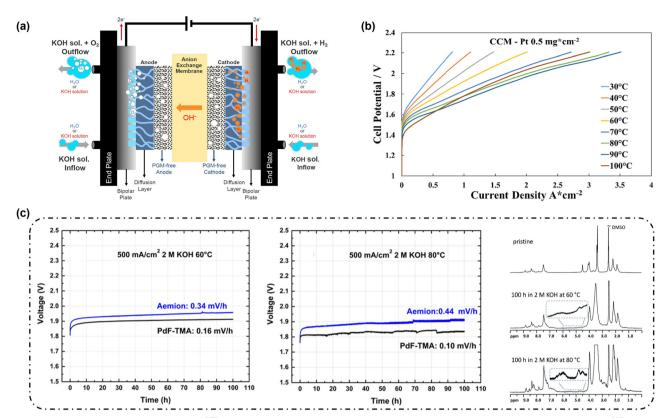
Fig. 23 (a) Schematic diagram of the AEMWE.<sup>257</sup> (b) Polarization curves for AEMWE on the CCM configuration at different temperatures.<sup>258</sup> (c) Stability evaluations at 500 mA cm<sup>-2</sup> in 2 M KOH at 60 °C and 80 °C and <sup>1</sup>H NMR spectra of the Aemion membrane before and after long-term stability evaluation in the electrolysis cell.<sup>259</sup>
