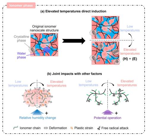
Fig. 11 Schemic diagram of ionomer degradation at elevated temperatures: (a) elevated temperature direct induction and (b) joint impacts with other factors
