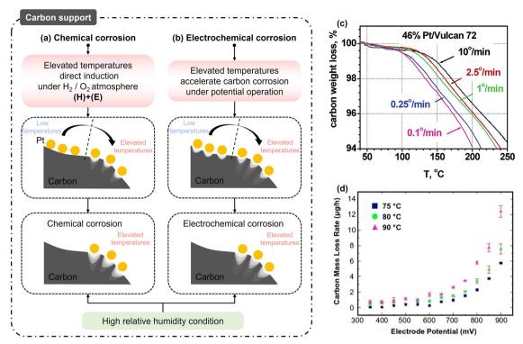
Fig. 10 Schemic diagram of carbon support corrosion at elevated temperatures: (a) chemical corrosion and (b) electrochemical corrosion. (c) TGA data for 46% Pt/C measured at heating rates of 0.1, 0.25, 1, 2.5, and 10 °C min<sup>-1.153</sup> (d) Decline in carbon content against the cell potential at varying temperatures.
