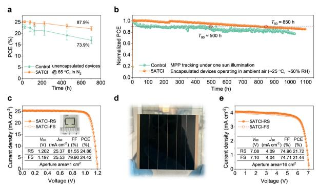
Fig. 5 Stability and scalability of PSCs. (a) Thermal stability of the unencapsulated PSCs with and without 5ATCI modification. (b) Operating stability of the encapsulated PSCs with and without 5ATCl modification. (c) J-V curves of the champion large-size PSCs with 5ATCl modification, with the inset showing the device picture. (d) The photograph and (e) J-V curve of the champion 5 cm  $\times$  5 cm mini-module with 5ATCl modification.
