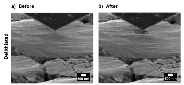
Fig. 4 Snapshots extracted from a real time video recorded during in situ nanoindentation testing showing the cross-section of NMC811 sample and the cube corner nanoindenter tip (a) prior to and (b) following the application of a 3 mN load. The sample was charged to 4.2 V vs. Li/Li<sup>+</sup> and disassembled in the delithiated state.
