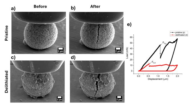
Fig. 2 The SEM images of NMC811 secondary particles before and after intragranular crack appearance in the pristine (a) and (b) and delithiated (c) and (d) states. The corresponding load-displacement curves (e) are presented with the critical loads denoted as  $F_{0,p}$  and  $F_{0,d}$  for pristine and delithiated particles respectively.
