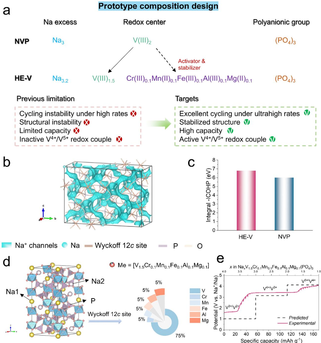
**Fig. 1** Composition design principle and theoretical studies of physicochemical properties. (a) Prototype composition design principle. (b)  $\text{Na}^+$  ion diffusion pathways (blue isosurface) in HE-V from the BV calculation. (c) Integral ICOHP values of all V–O bonds in HE-V and NVP. (d) Illustrations of crystalline structures and transition metal compositions in HE-V. (e) Calculated voltage profile.
