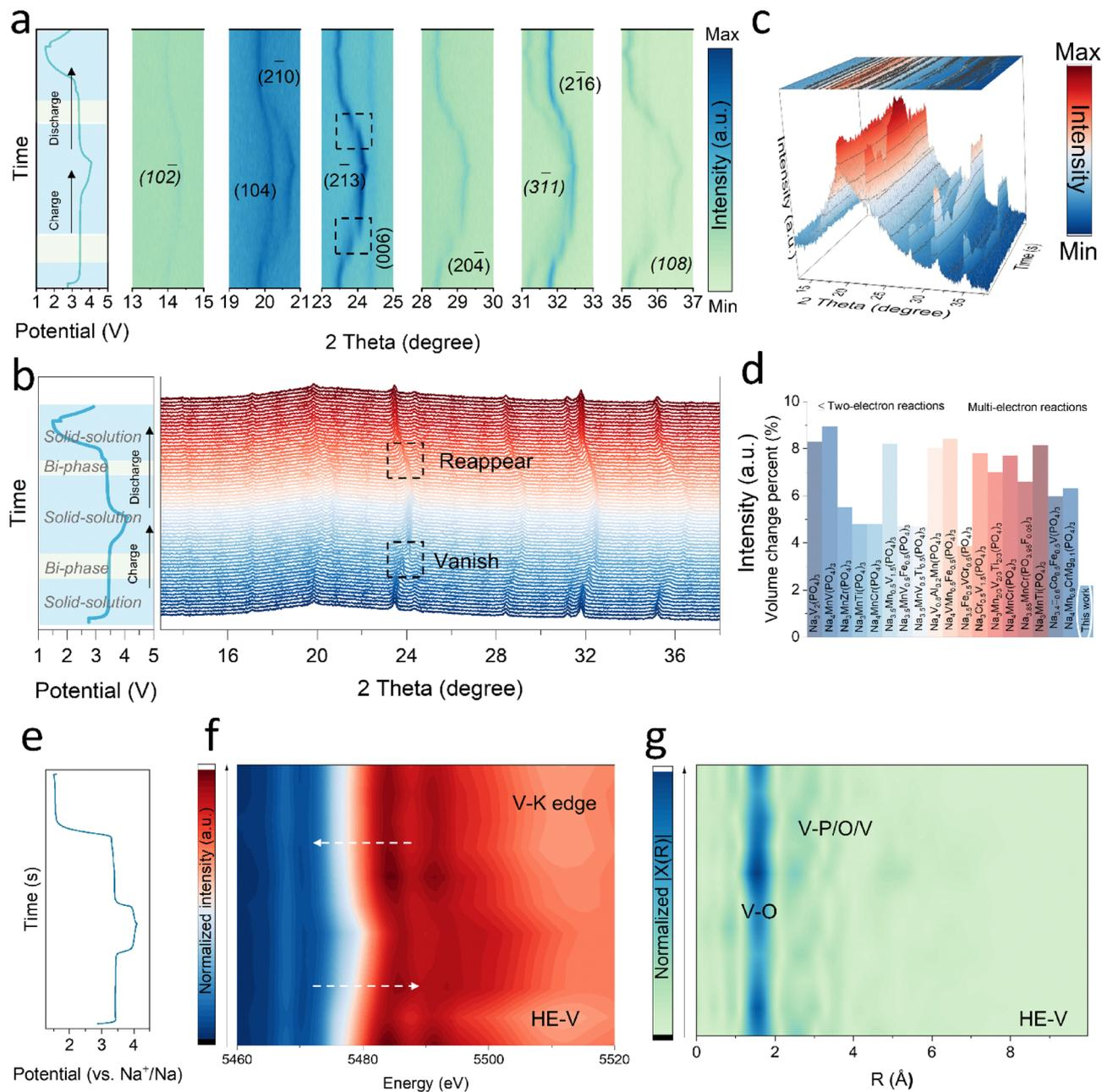
Fig. 4 Structural evolution and charge compensation analysis. (a)–(c) *In situ* XRD patterns of HE-V. (d) A volumetric change comparison of HE-V and reported NASICON cathodes upon battery operation. (e) The galvanostatic charge–discharge curve and (f) XANES spectra at different charging states as a function of the V K-edge of the HE-V electrode (2D contour plot) and (g) corresponding  $k^2$ -weighted Fourier transform magnitudes of HE-V.
