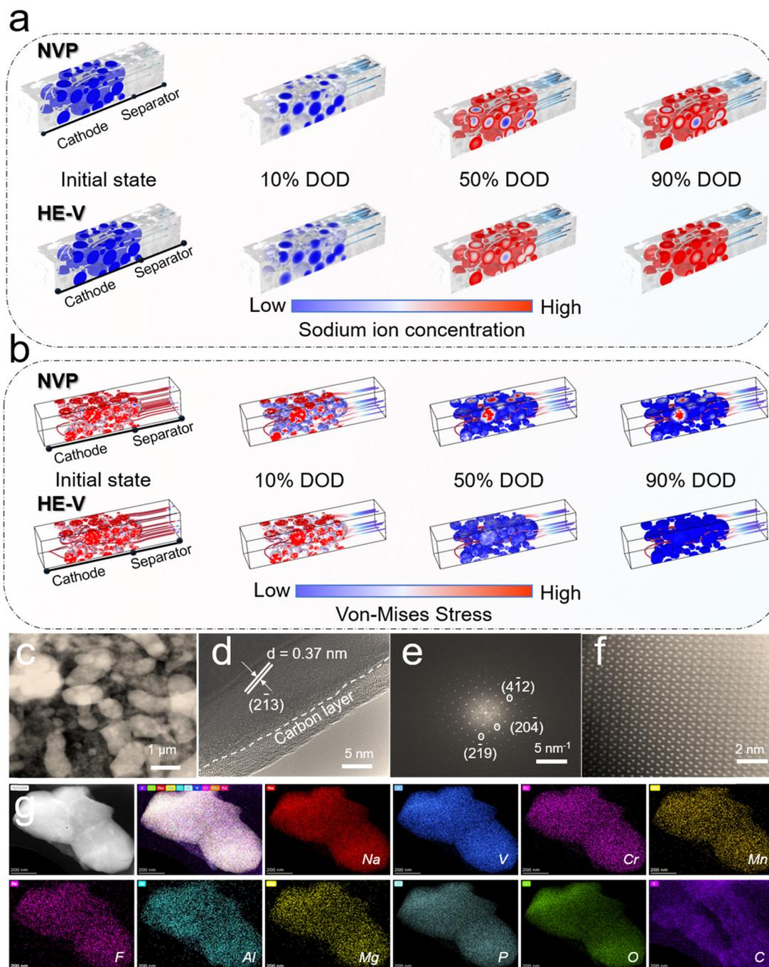
Fig. 5 COMSOL simulation and postmortem analysis. (a)  $\text{Na}^+$  distribution and (b) stress field analysis at different depths of discharge (DOD) states based on the COMSOL platform. Postmortem analysis of the cycled HE-V: (c) TEM, (d) HRTEM, (e) FFT, and (f) aberration-corrected STEM image. (g) EDS mapping images.
