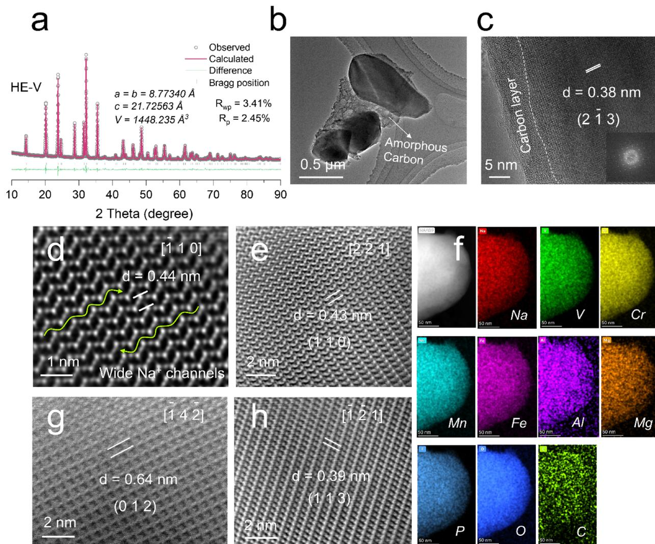
Fig. 2 Material characterization of HE-V. (a) XRD Rietveld refinement results. (b) and (c) TEM and HRTEM images. (d)–(h) Aberration-corrected STEM images viewed from the (d)  $[1\bar{1}0]$ , (e)  $[22\bar{1}]$ , (g)  $[1\bar{4}2]$ , and (h)  $[1\bar{2}1]$  crystallographic directions. (f) EDS mapping images (scale bar: 50 nm).
