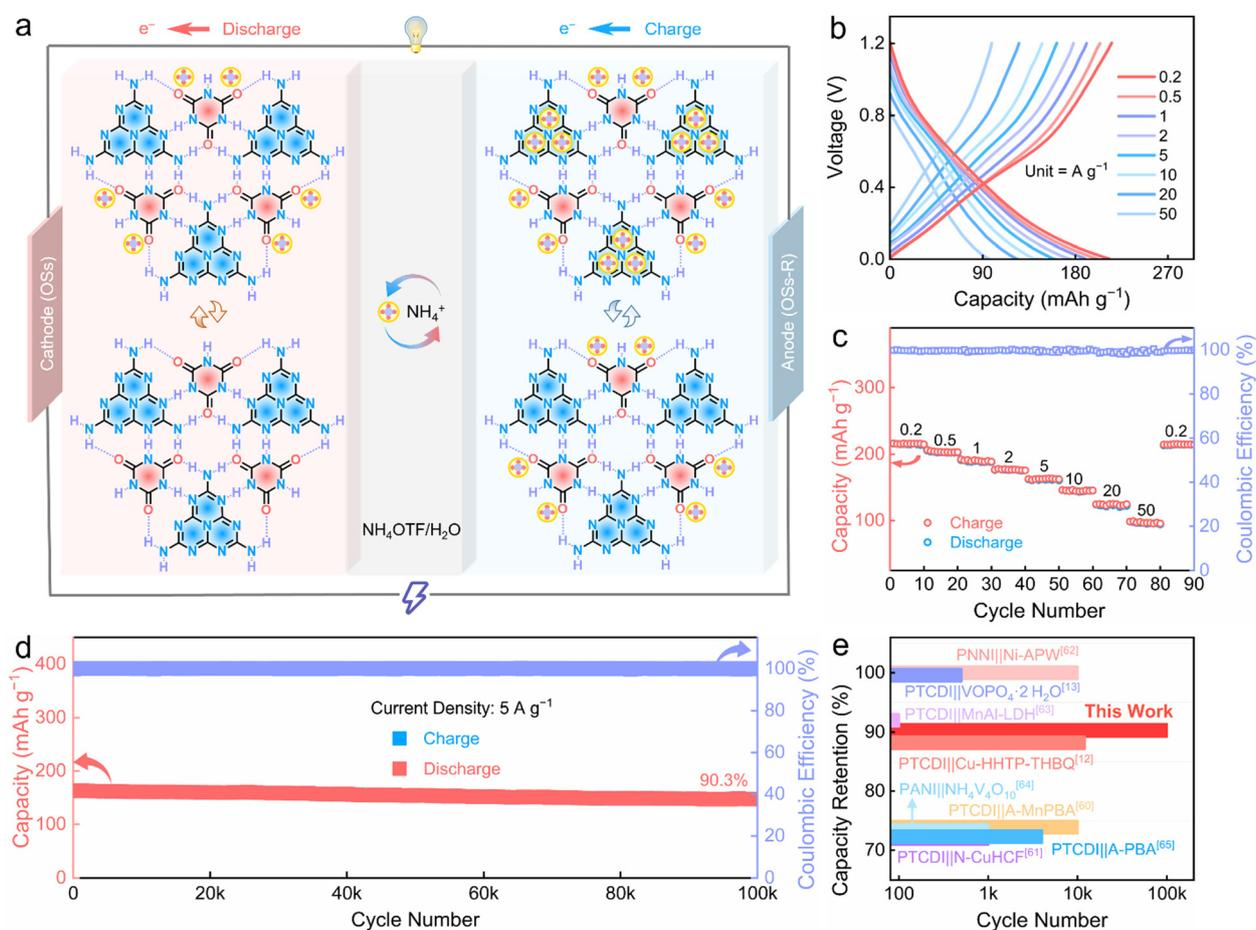
Fig. 5 Electrochemical evaluation of AOBs. (a) Schematic of the OSs||OSs-R cell. (b) GCD curves. (c) Rate metrics. (d) Long-term cycling performance. (e) Lifespan comparison with reported  $\text{NH}_4^+$ -ion full cells.
