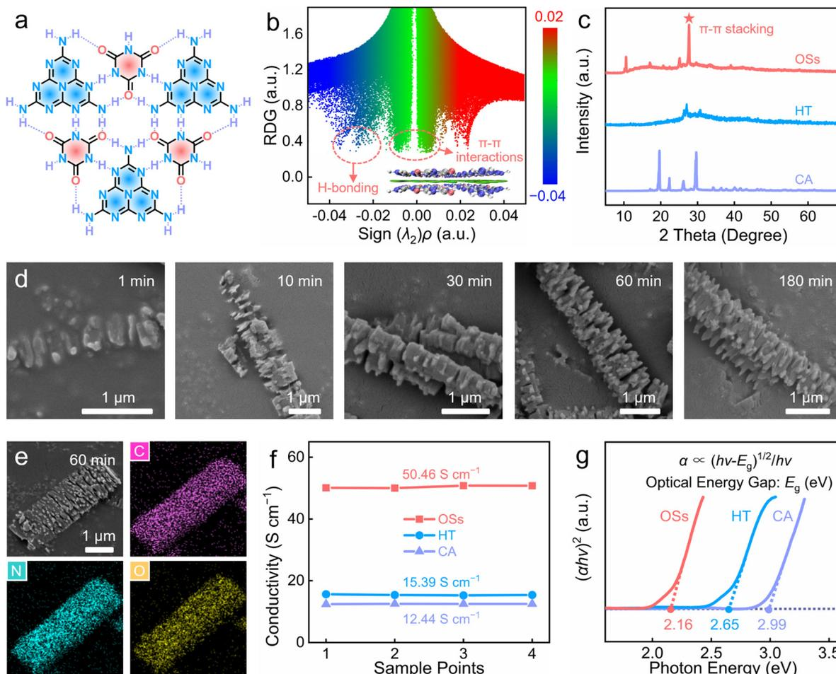
**Fig. 1** Structural characterization of the OSs. (a) Two-dimensional supramolecular planar structure interconnected by multiple interlocking hydrogen bonds between CA and HT. (b) RDG map and corresponding isosurface. (c) XRD patterns. (d) SEM images recorded at different reaction times. (e) Elemental maps. (f) Electrical conductivities. (g)  $E_g$  values.
