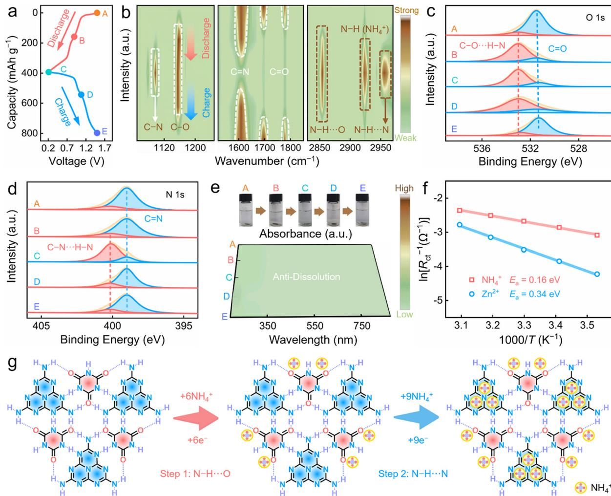
Fig. 3 Structural evolution of the OSs cathode during (dis)charging. (a) Voltage-capacity curve measured at  $0.2 \text{ A g}^{-1}$ . (b) *Ex situ* FT-IR spectra. (c) O 1s and (d) N 1s XPS spectra. (e) UV/vis spectra and images of the OSs cathodes in  $\text{NH}_4\text{OTf}/\text{H}_2\text{O}$  electrolytes at various electrochemical states. (f) Calculated  $E_a$  values. (g) H-bonding redox chemistry.
