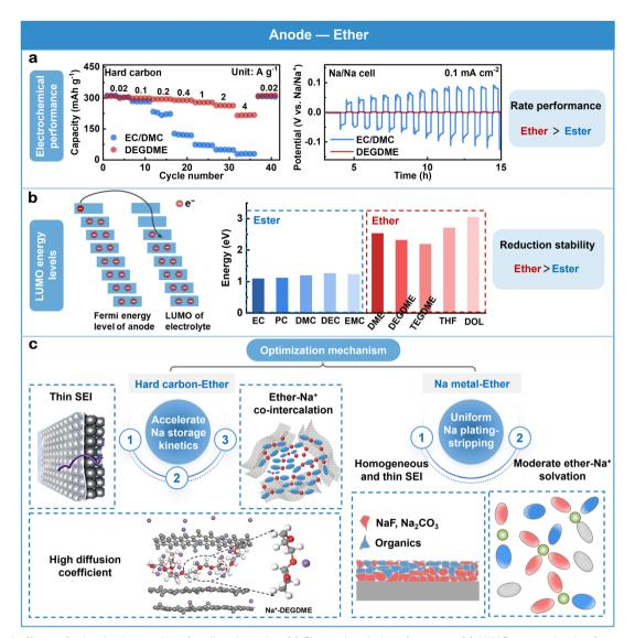
Fig. 7 Critical effects of ether in the anodes of sodium batteries. (a) Electrochemical performance. (b) LUMO energy levels of esters and ethers. (c) Optimization mechanism of ether on HC and Na metal anodes.
