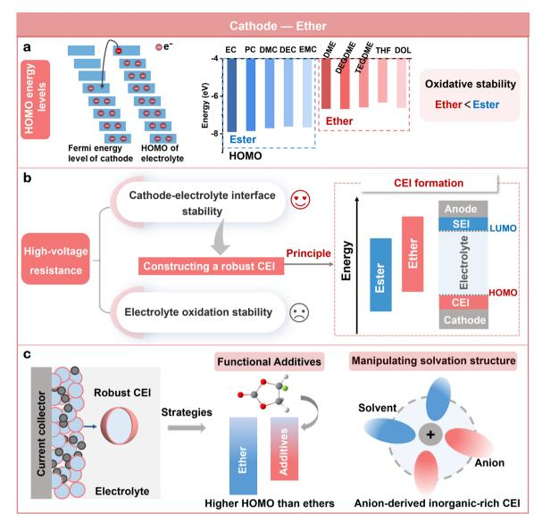
Fig. 10 Critical effects of ethers in the cathodes of sodium batteries. (a) HOMO energy levels of esters and ethers. (b) Optimization mechanism of ethers on cathodes. (c) Strategies for forming a robust CEI.
