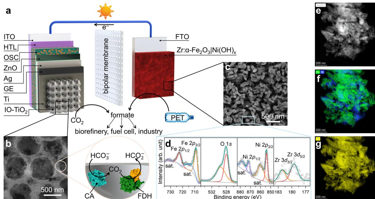
**Fig. 1** (a) Schematic illustration of the organic–inorganic PEC tandem device. (b) Top-view SEM image of IO-TiO<sub>2</sub> with illustration of co-immobilisation of FDH (PDB: 6sdv) and CA (PDB: 1v9e). (c) Top-view SEM image, (d) XPS spectra, (e) HAADF image, and TEM elemental mapping for (f) Fe (green), Ni (blue), and (g) O (yellow) of Zr:α-Fe<sub>2</sub>O<sub>3</sub>|Ni(OH)<sub>x</sub>.
