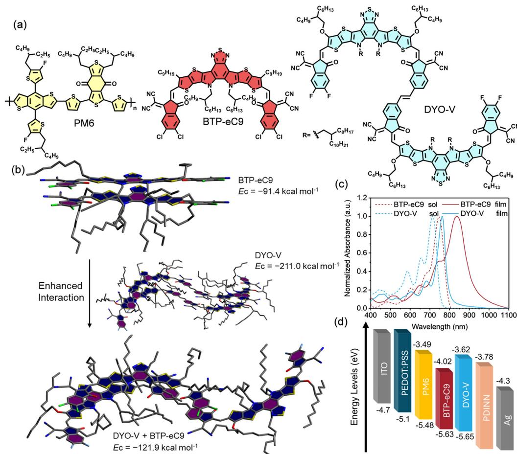
**Fig. 1** (a) Chemical structures of PM6, BTP-eC9 and DYO-V. (b) Non-covalent interaction energies of BTP-eC9/BTP-eC9, DYO-V/DYO-V and BTP-eC9/DYO-V obtained from MD simulations and DFT calculations. (c) Normalized UV-Vis absorption spectra of the BTP-eC9 and DYO-V in the chloroform solution and the neat film state. (d) Energy alignment of the materials and device structure in OSCs.
