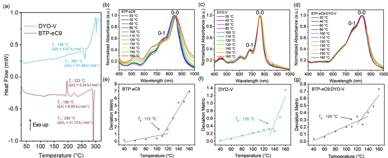
Fig. 2 (a) DSC thermograms of BTP-eC9 and DY0-V, collected from the first cycle with a  $10^\circ\text{C min}^{-1}$  heating rate. (b)–(d) Temperature-dependent absorption spectra and (e)–(g) deviation metrics obtained from the temperature-dependent absorption of the BTP-eC9, DY0-V and BTP-eC9:DYO-V films.
