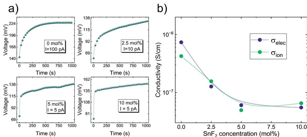
Fig. 2 (a) Galvanostatic polarization curves from  $\text{FASn}_{0.5}\text{Pb}_{0.5}\text{I}_3$  samples with different  $\text{SnF}_2$  concentrations: 0, 2.5, 5, and 10 mol% (b)  $\sigma_{\text{elec}}$  and  $\sigma_{\text{ion}}$  as a function of  $\text{SnF}_2$  concentration.
