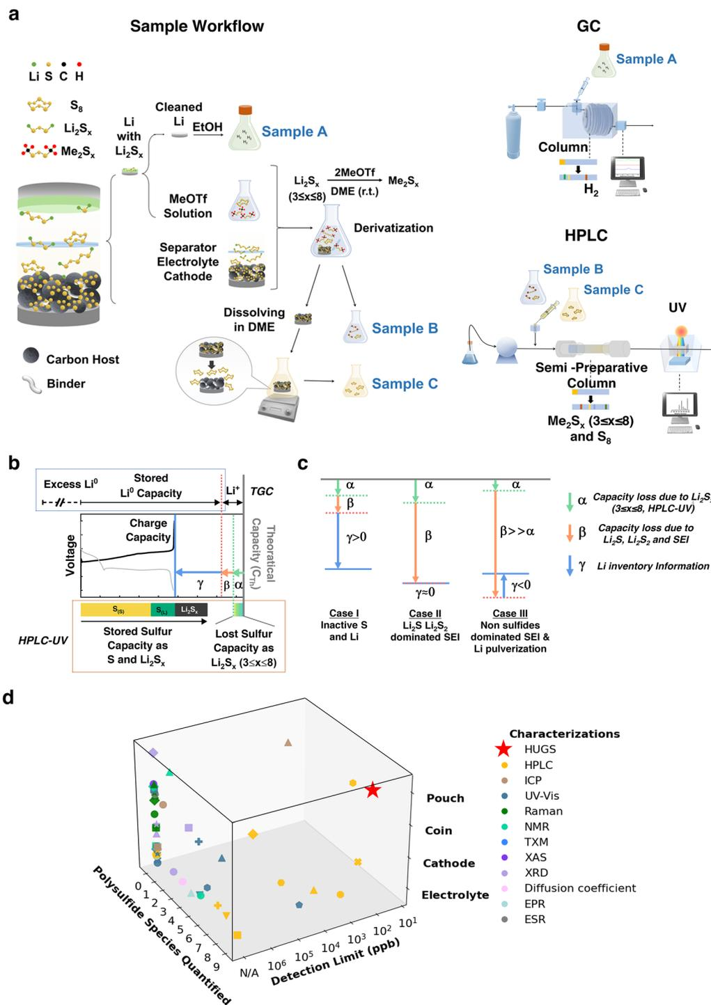
**Fig. 1** HUGS method sample preparation and results interpretation. (a) Schematic of HUGS; (b) information output based on HUGS; (c) three capacity loss mechanism scenarios in Li-S battery derived from HUGS; (d) 3D scatter plot comparing bulk characterization methods based on the quantification of polysulfide species, their detection limits, and the system in which the method was tested.
