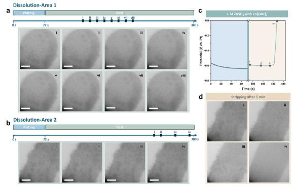
Fig. 5 In situ liquid cell TEM imaging of the dissolution of plated Zn deposits in  $ZnSO_4$  electrolyte with  $Zn(OAc)_2$ : (a) area 1 and (b) area 2. Scale bars are 1  $\mu$ m. (c) Corresponding galvanostatic voltage profile of plating and stripping after rest for 5 minutes. (d) In situ liquid cell TEM imaging of the stripping process after rest for 5 minutes. Scale bars are 1  $\mu$ m.
