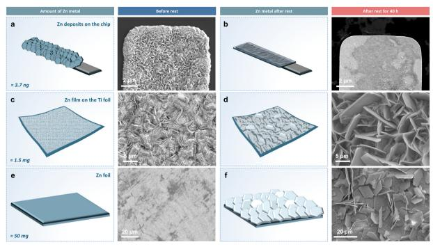
Fig. 4 Schematic illustrations and SEM images of electrodes with increasing quantity of Zn metal before and after resting in a 1 M ZnSO<sub>4</sub> electrolyte vial for 40 hours. (a) and (b) Zn deposited to 1 mA h cm<sup>-2</sup> on a liquid cell TEM chip Pt electrode (approximately 3.7 ng of Zn). (c) and (d) A thin Zn film deposited on a Ti foil electrode (approximately 1.5 mg of Zn). (e) and (f) Zn foil electrode (approximately 50 mg of Zn).
