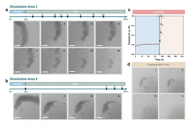
Fig. 3 In situ liquid cell TEM imaging of the dissolution of Zn deposits during cell rest in the ZnSO<sub>4</sub> electrolyte for (a) area 1 and (b) area 2. Scale bars are 1 µm. (c) Corresponding galvanostatic voltage profile. (d) In situ liquid cell TEM imaging of the stripping process after rest for 5 minutes. Scale bars are 1 µm.
