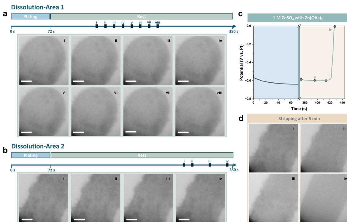
Fig. 5 *In situ* liquid cell TEM imaging of the dissolution of plated Zn deposits in  $\text{ZnSO}_4$  electrolyte with  $\text{Zn}(\text{OAc})_2$ : (a) area 1 and (b) area 2. Scale bars are  $1 \mu\text{m}$ . (c) Corresponding galvanostatic voltage profile of plating and stripping after rest for 5 minutes. (d) *In situ* liquid cell TEM imaging of the stripping process after rest for 5 minutes. Scale bars are  $1 \mu\text{m}$ .
