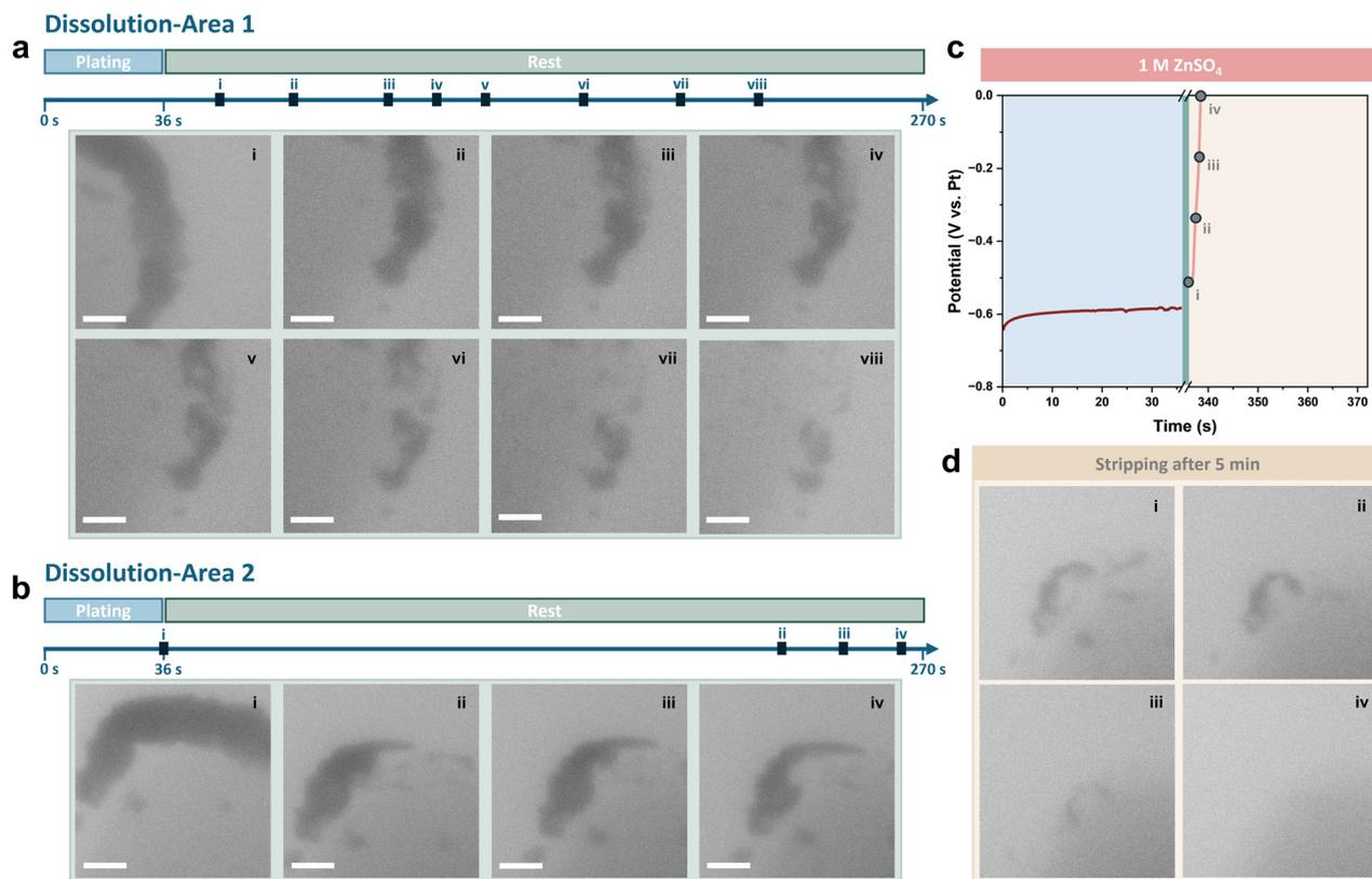
Fig. 3 *In situ* liquid cell TEM imaging of the dissolution of Zn deposits during cell rest in the  $\text{ZnSO}_4$  electrolyte for (a) area 1 and (b) area 2. Scale bars are  $1 \mu\text{m}$ . (c) Corresponding galvanostatic voltage profile. (d) *In situ* liquid cell TEM imaging of the stripping process after rest for 5 minutes. Scale bars are  $1 \mu\text{m}$ .
