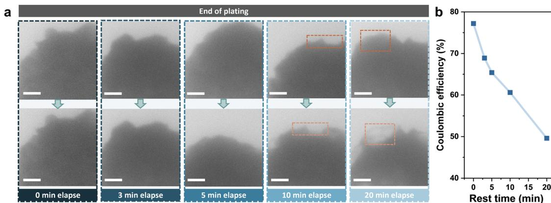
Fig. 2 (a) *In situ* liquid cell TEM images of the end of plating before and after rest for different periods of time. Scale bars are 1  $\mu$ m. (b) The corresponding coulombic efficiency after rest for different periods of time.
