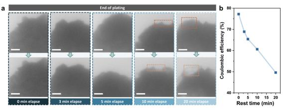
Fig. 2 (a) In situ liquid cell TEM images of the end of plating before and after rest for different periods of time. Scale bars are 1 μm. (b) The corresponding coulombic efficiency after rest for different periods of time
